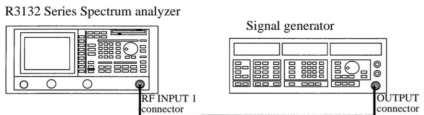
**Figure 2-27 Setup for Verifying the Dynamic Range**
