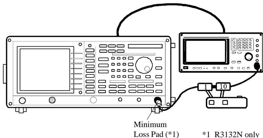
**Figure 5-7 Setup of IF Gain Uncertainty Test**
