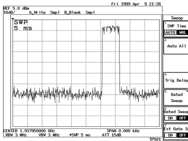
Figure 2-74 Burst Signal in the Time Domain
