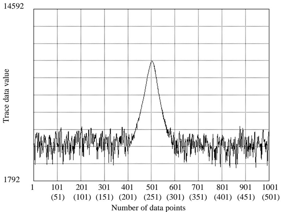
**Figure 4-4 Relationship between Screen Graticule and Trace Data**
