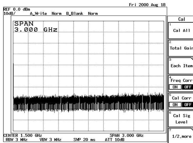
Figure 2-42 Screen Display Showing the Cal Menu
