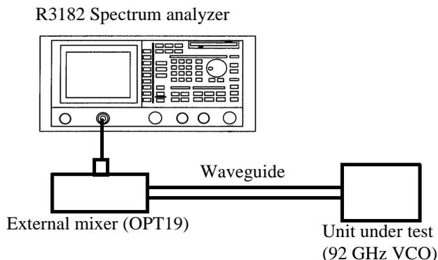
**Figure 2-94 Setup for measuring VCO Output Levels**
