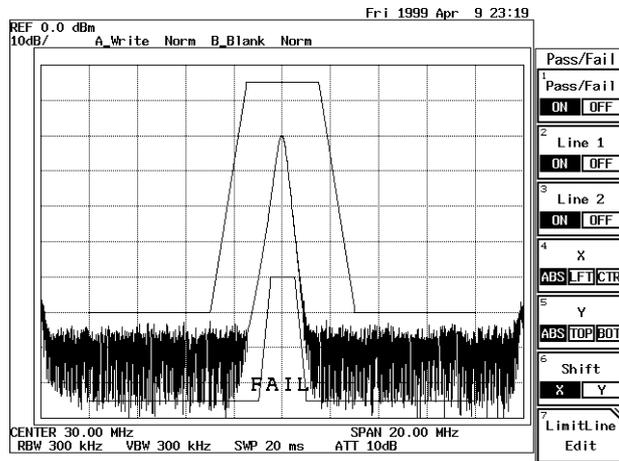
Figure 2-81 PASS/FAIL Result using Limit Lines 1 and 2 (FAIL)
