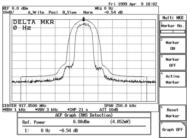
Figure 2-60 Measurement Using ACP GRAPH
