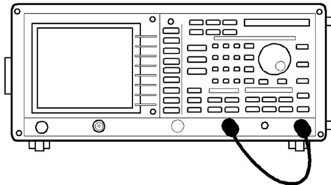
**Figure 5-4 Setup of Resolution Bandwidth Switching Uncertainty**
