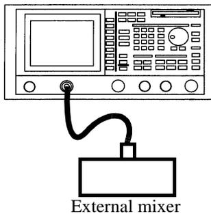
Figure 2-47 Setup for the R3182 and Waveguide Mixer
