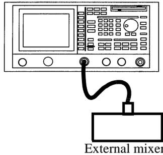
Figure 2-46 Setup for the R3172 and Waveguide Mixer
