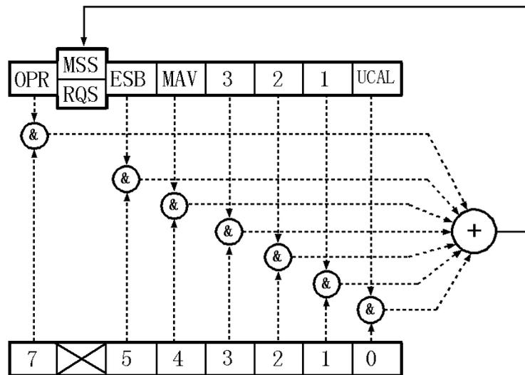
**Figure 4-3 Structure of the Status Byte Register**
