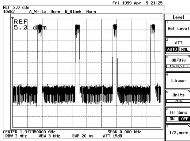
Figure 2-73 Burst Signal in the Time Domain
