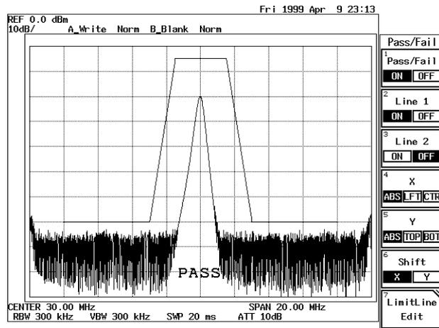
Figure 2-80 PASS/FAIL Result using Limit Line 1 (PASS)
