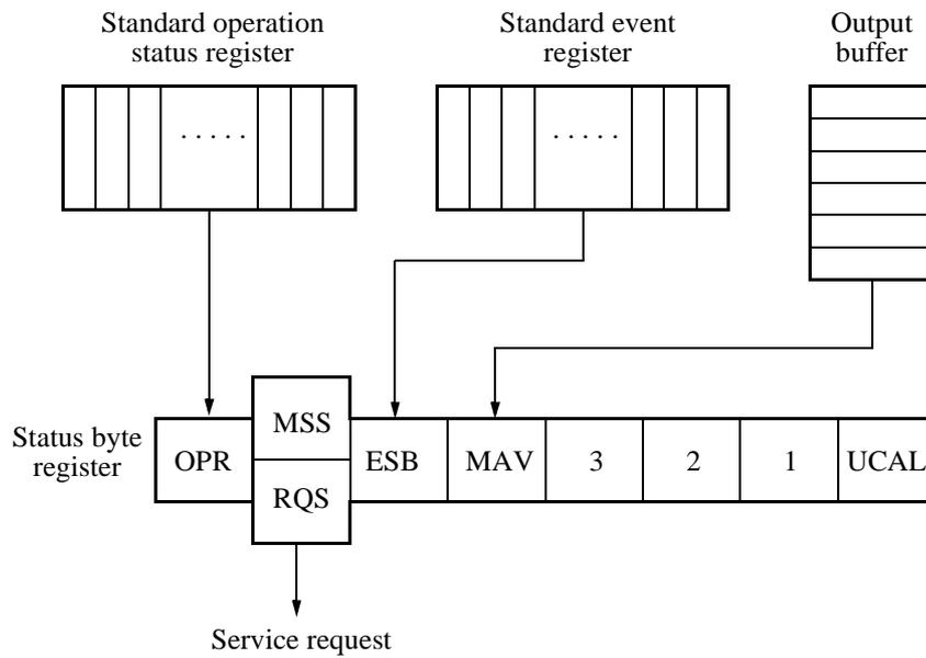
**Figure 4-1 Arrangement of the Three Status Registers**
