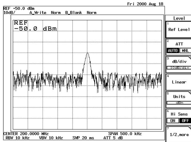
Figure 2-28 Screen Display Prior to Changing the RBW
