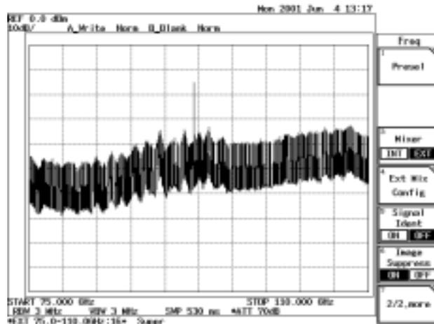
Figure 2-96 Measurement Signal with the Image Signal Eliminated
