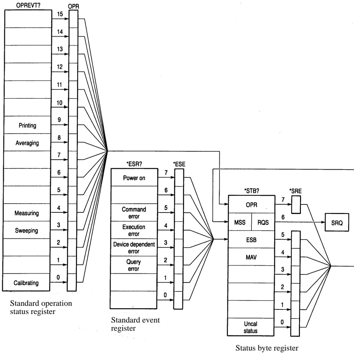
Figure 4-2 Details of the Three Status Registers
