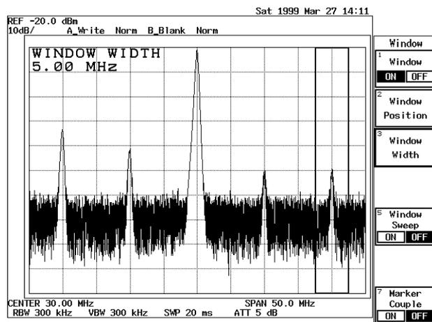
**Figure 2-13 Screen Display Showing the Measuring Window**
