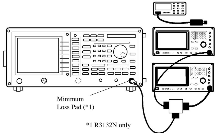
**Figure 5-18 Setup of Third Order Intermodulation Distortion Test**
