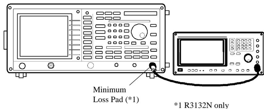
**Figure 5-20 Setup of Sweep Time Accuracy Test**
