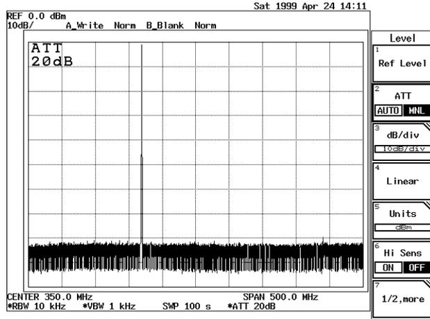
**Figure 2-38 Screen Display Showing Reduced Harmonic Distortion**
