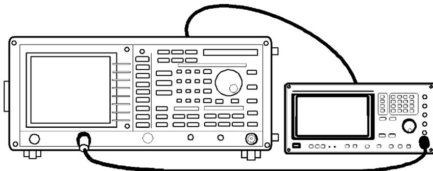
**Figure 5-31 Setup for Checking the Linearity Error (External Mixer Mode)**
