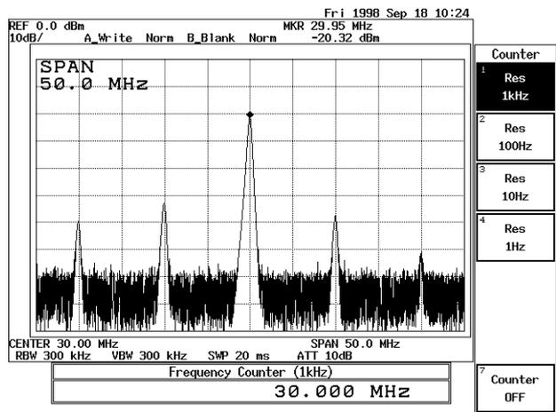
Figure 2-15 Frequency Counter Measurement (Resolution: 1 kHz)
