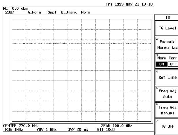
Figure 2-86 Measurement Screen after a Normalization Calibration
