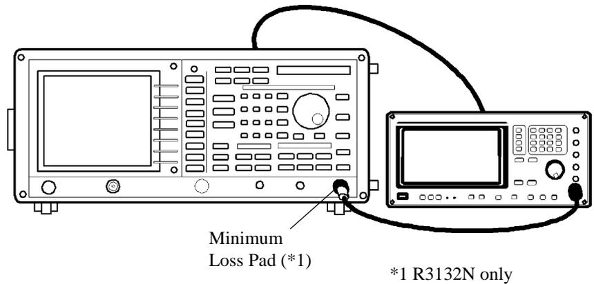
**Figure 5-17 Setup of Frequency Span Accuracy Test**
