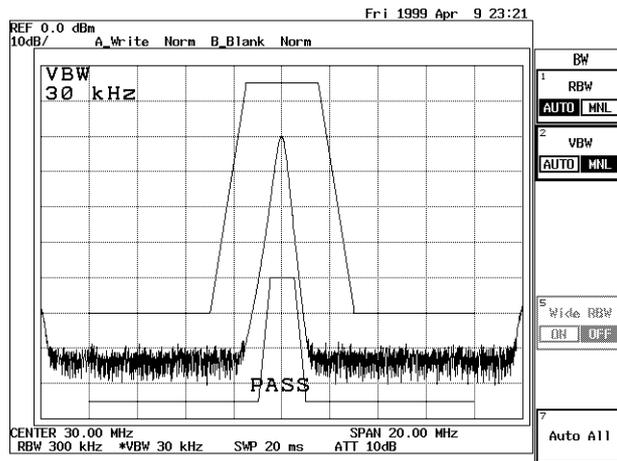
Figure 2-82 PASS/FAIL Result using Limit Lines 1 and 2 (PASS)
