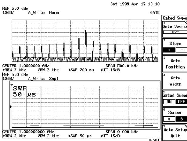
Figure 2-67 Burst Signal Displayed in Split Screen Mode
