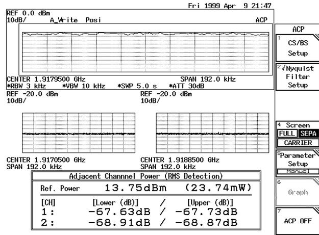
Figure 2-65 Measurement Result in ACP Separate Screen Mode
