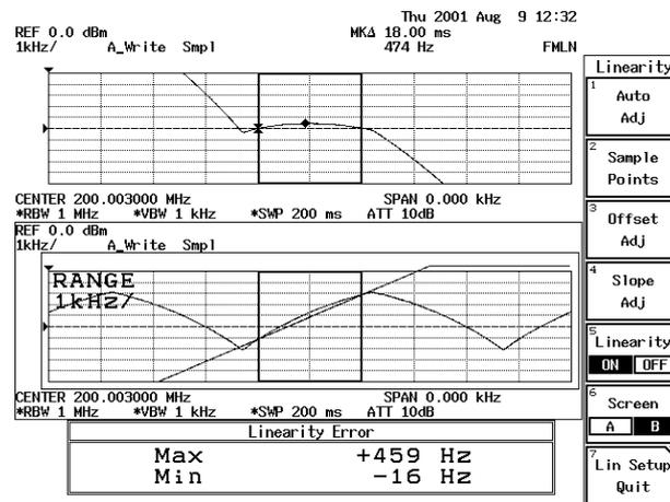
Figure 2-105 Linearity Measurement
