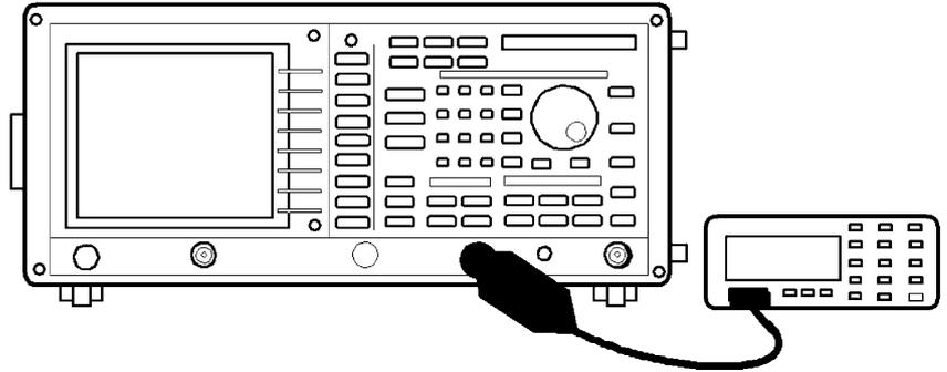
**Figure 5-2 Setup of CAL OUT Level Accuracy Test**
