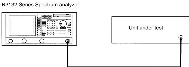
**Figure 2-51 Setup for Measuring the Occupied Bandwidth**
