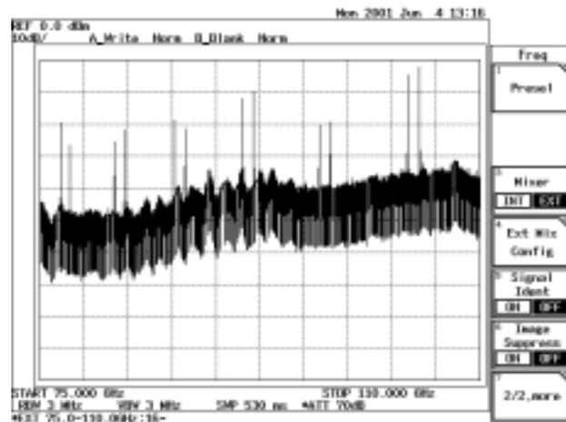
Figure 2-95 Measurement Signal with an Image Signal
