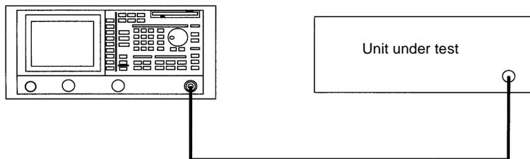
**Figure 2-62 Setup Measuring Adjacent Channel Leakage Power**
