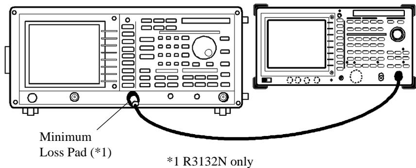
**Figure 5-26 Setup of Non Harmonic Distortion Test**
