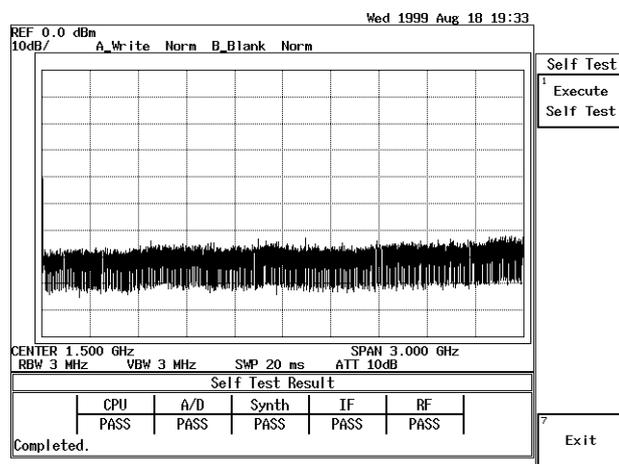
**Figure 1-7** Screen Shown after Executing Self Test
