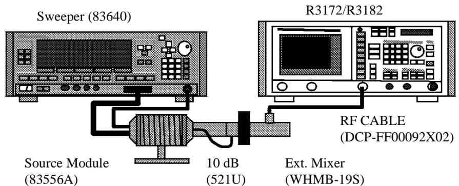
**Figure 6-4 Setup of Noise Level Test**
