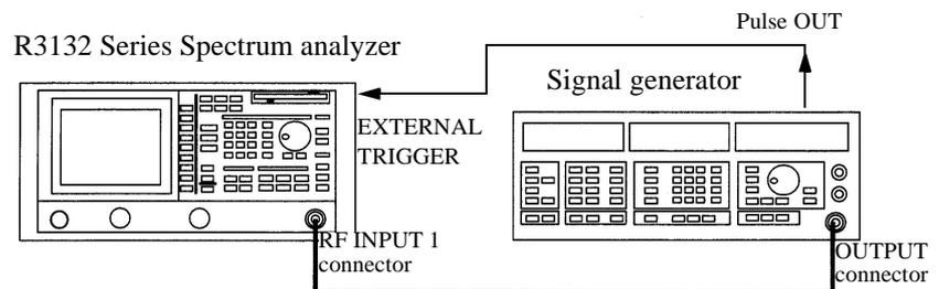
**Figure 2-66 Setup for Measuring a Burst Signal**
