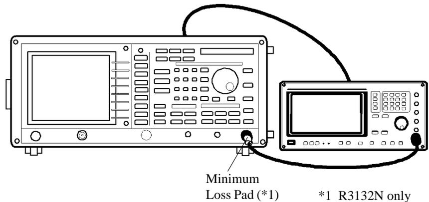
**Figure 5-11 Setup of Residual FM Test**
