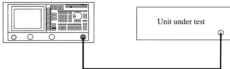
**Figure 2-90 Setup for Measuring the Spectrum Mask**
