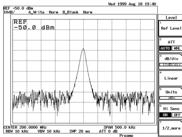
Figure 2-32 Spectrum Displayed when the pre-amplifier is Used
