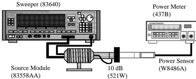
**Figure 6-11 Setup of Source Module Calibration**
