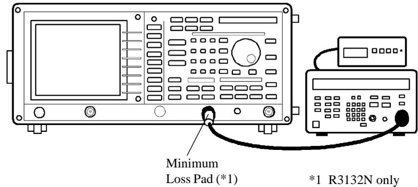
**Figure 5-1 Setup of Frequency Reference Source Accuracy Test**
