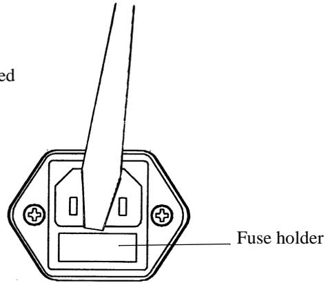
Check (and replace if necessary) the power fuse and put it back into the fuse holder.
