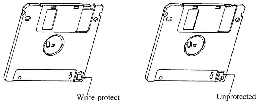
**Figure 2-106 Floppy Disk Write Protection**
