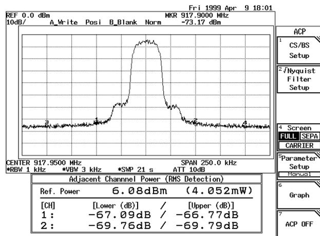
Figure 2-59 ACP Measurement Display in Full Screen Mode
