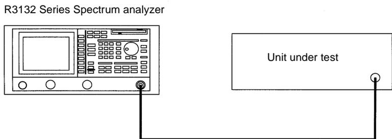
**Figure 2-55 Setup Measuring Adjacent Channel Leakage Power**
