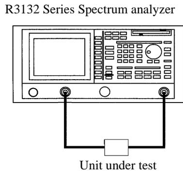
**Figure 2-87 Connecting the Unit under Test**
