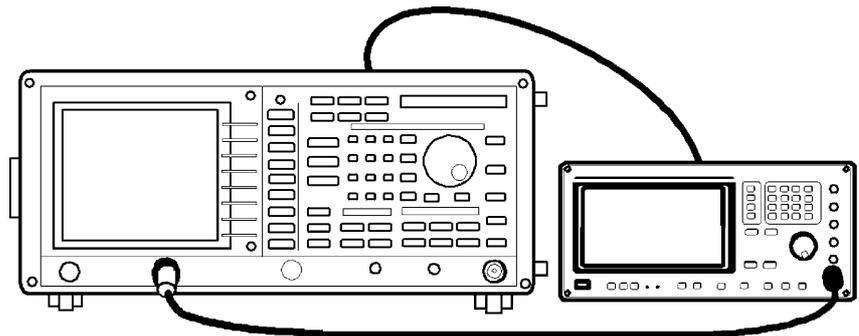
**Figure 5-30 Setup for Checking the Offset Error (External Mixer Mode)**
