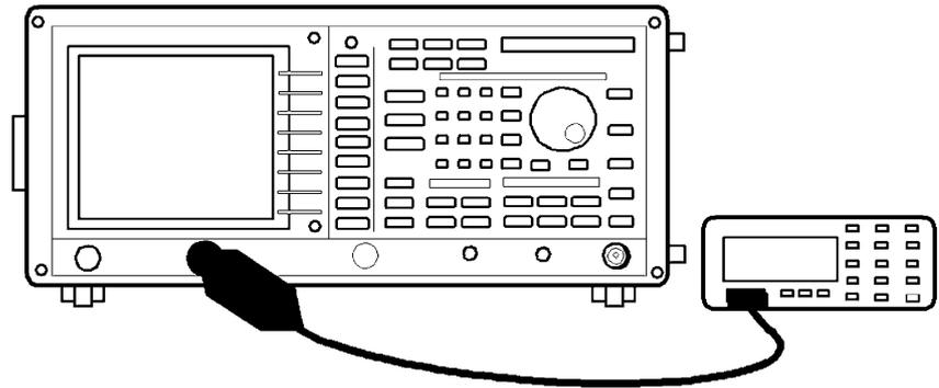
**Figure 5-23 Setup of Output Level Flatness Test**
