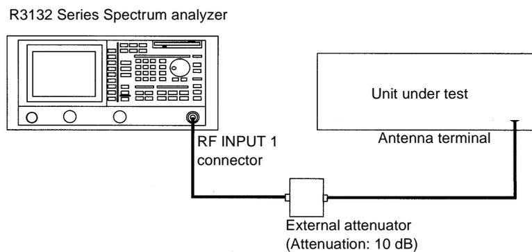
**Figure 2-48 Setup for Measuring the Channel Power**
