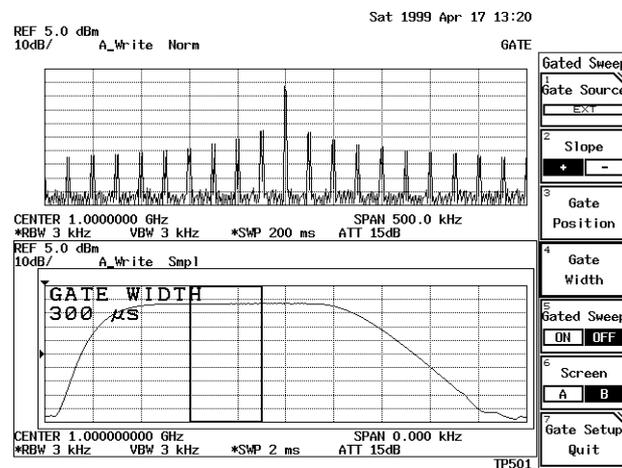
Figure 2-69 Gate Setup
