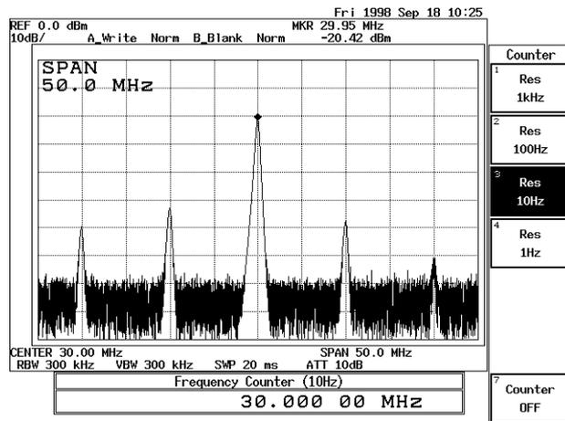
**Figure 2-16 Frequency Counter Measurement (Resolution: 10 Hz)**
