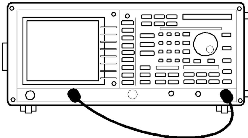
**Figure 5-24 Setup of Output Switching Accuracy Test**
