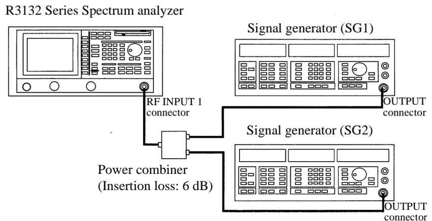
**Figure 2-33 Setup for Input Saturation**
