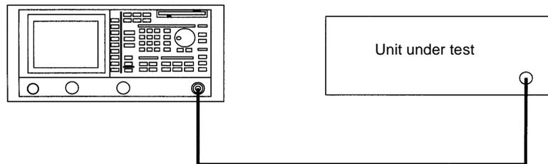
**Figure 2-72 Setup for Measuring a Burst wave signal**
