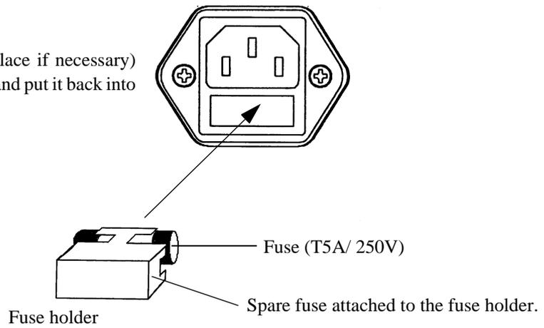
**Figure 1-2 Replacing the Power Fuse**
