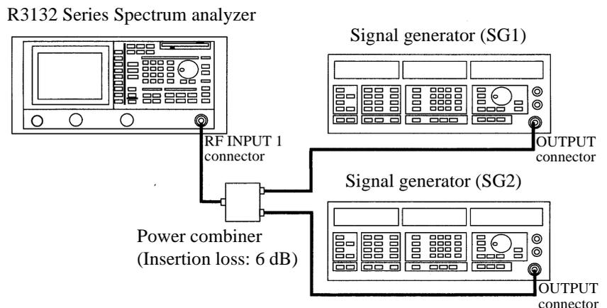
**Figure 2-39 Setup for Measuring Intermodulation**
