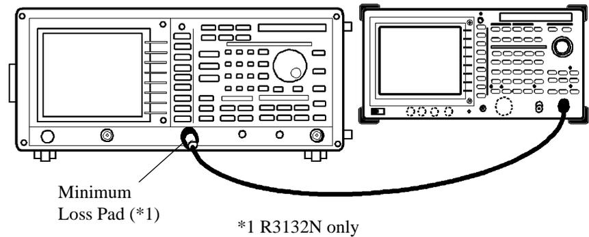
**Figure 5-25 Setup of Harmonic Distortion Test**
