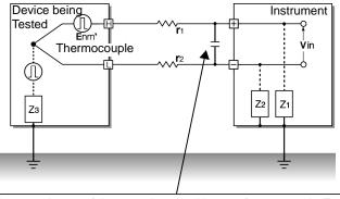
The capacitance of the capacitor should range from several  $\mu F$  to several thousand  $\mu F.$  Insert the capacitor between the "+" and "-" input terminals.
