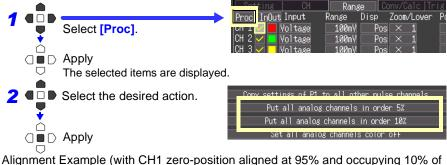
Alignment Example (with CH1 zero-position aligned at 95% and occupying 10% of vertical screen height)
