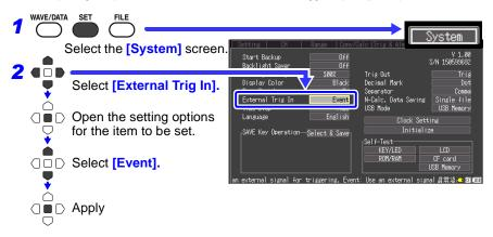
Connect the external signal input (p. 157).
