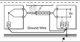
If the signal side is not grounded or if it is grounded inadequately, connect the instrument to ground. Also ground the shielding for the signal wires on the instrument side securely.
