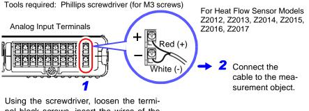
nal block screws, insert the wires of the cable as shown in the figure and tighten the screws.
