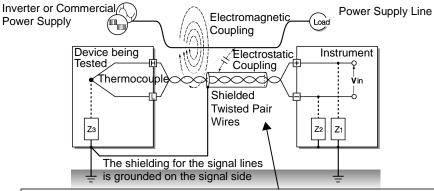
Keep the signal lines (of the thermocouple) away from wiring that is a noise source (such as power lines, etc.). It is also possible to shield the signal lines from electrostatic coupling and to block noise by grounding the shield.
