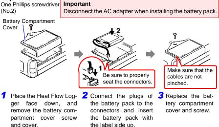
Pull the battery pack plug straight out to remove the battery pack.
