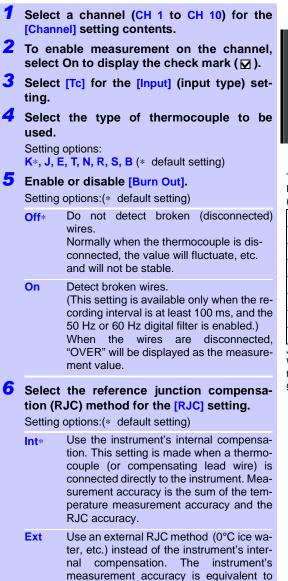
the temperature measurement accuracy.
