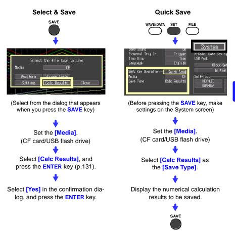
By specifying a particular time span for numerical calculation, only the results for that time span are saved.
