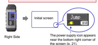
If the icon " **[1]**" is not displayed, the instrument is not being powered from the AC line. In this state, the battery charge will be depleted if measuring for a long time, and measurement may be interrupted. Verify that the AC adapter is securely connected to an AC power source and to the instrument.
