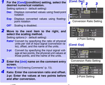
**NOTE** Scaling (voltage [V] to heat flow [W/m<sup>2</sup>]) is automatically set when the sensitivity constant is set during heat flow measurement. (p. 61)
