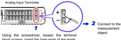
block screws, insert the bare ends of the leads, and tighten the screws.
