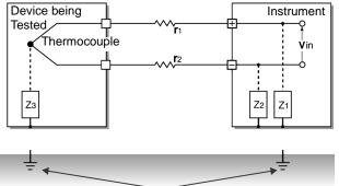
When using a thermocouple to measure temperature, noise can affect measurements unless both the device being tested and the instrument are grounded. Although there is no problem if the instrument is running on battery power, the instrument must be connected to ground if an AC adapter is being used.
