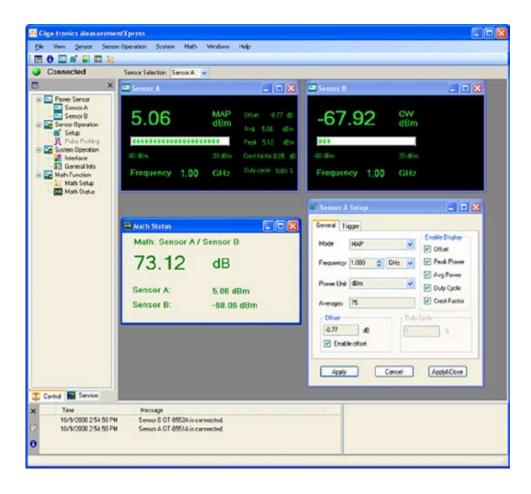
The Giga-tronics GT-8550A series USB Power Sensors are designed for fast measurement speed, wide dynamic range and high accuracy. The unique circuit topology is highly reliable, with performance that excels where extremes of measurement speed and accuracy are required. The PC based platform allows for lower cost than traditional power meters and power sensors, and with a laptop PC is ideal for field portable power measurement or remote monitoring applications.
