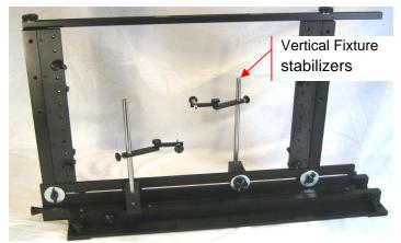
**Left)** GP2-35-R-12AR-VM 12 axis manipulator probing PCB held in V-PCB-REC-19 Vertical fixture. **Top)** Fount view of Vertical fixture that holds 2x2" to 19" PCB's which contain front and back side stabilizers, preventing PCB from flexing while probing.
