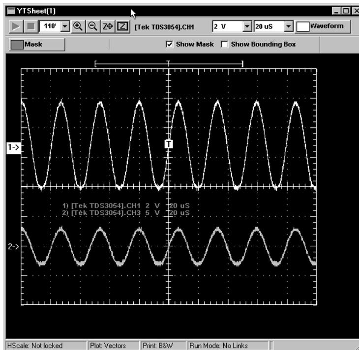
**Copying Waveforms To and From an Instrument.**
