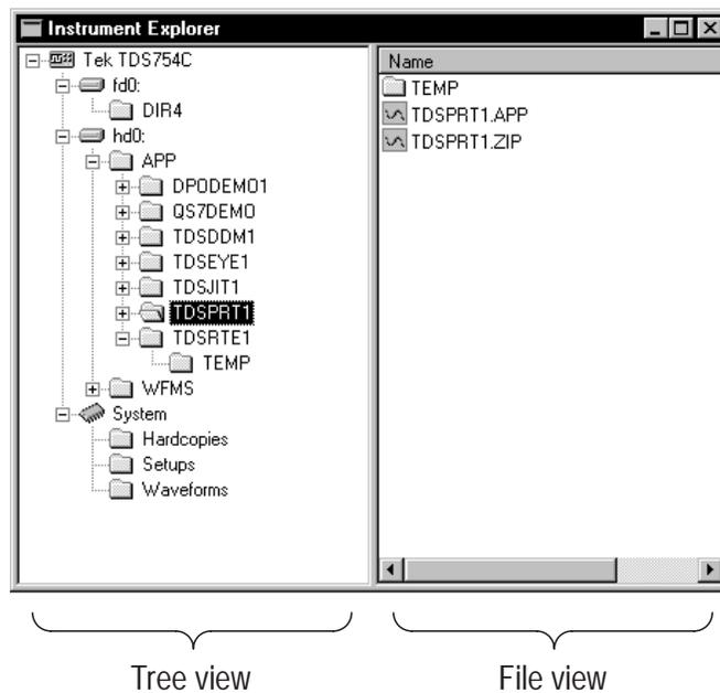
The Instrument Explorer sheet consists of a tree view and a file view. The tree view (left side) shows drive directories and subdirectories in a hierarchical tree layout, as well as instrument system files such as saved setups and waveforms. The files view (right side) shows the contents of a selected tree view directory.
