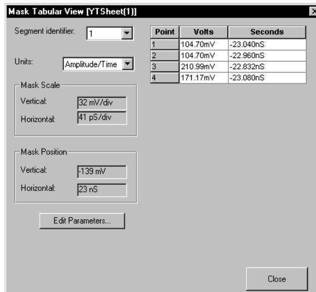
To edit the values in the dialog box, position the cursor in the table cell to edit, then left-click the mouse. Enter the new value for the cell. Repeat for each cell to edit. The mask segment updates immediately when you enter new values in the table.
