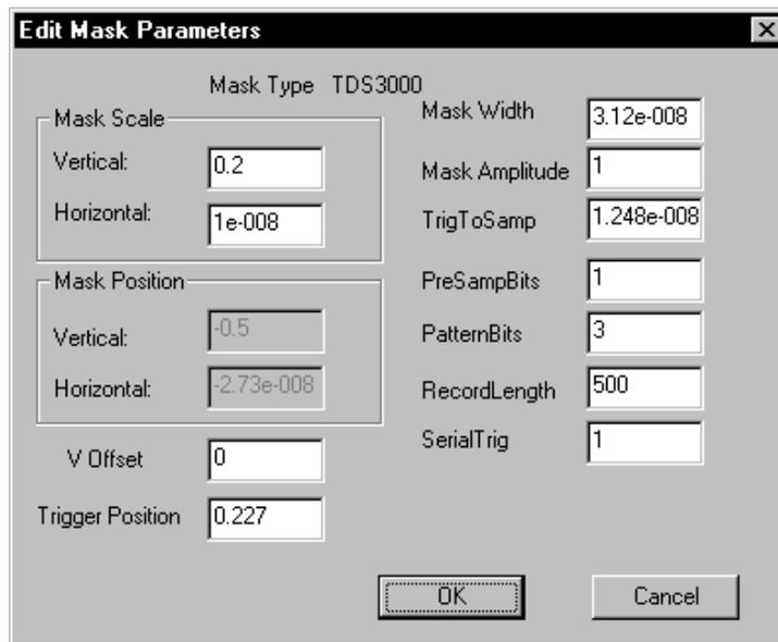
**Saving a Mask.** WaveStar handles a YT sheet with a mask just like any other data sheet file; you can save the YT sheet as part of a workbook, or you can save the YT sheet to an individual file. You can create a mask library by creating a workbook that contains only YT sheets with mask data. You can also save mask data by exporting it to a .MSK format file. Refer to page 4–42 for information on how to import and export .MSK files.
