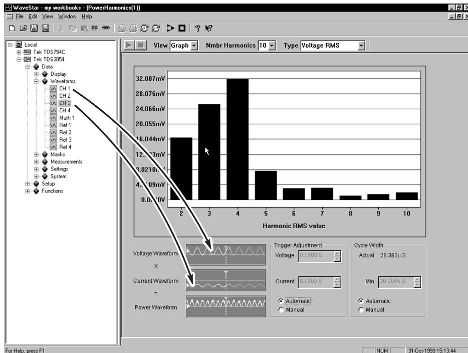
Once both waveforms are copied or linked, the Power Harmonics sheet calculates the power waveform by multiplying the voltage and current waveforms. You can copy or link the calculated power waveform to another data sheet. WaveStar recalculates and updates power and harmonic information whenever the data changes (when linked) or a refresh action occurs.
