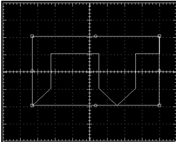
**Moving Mask Segment Points.** To select a segment point, position the cursor on the point. A selected point fills with the current mask color. To move the point, press and hold the left mouse button and drag the point to a new location.
