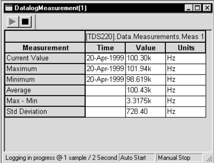
The screenshot shows a window titled "DatalogMeasurement(1)" with a table of measurement statistics. The table has four columns: Measurement, Time, Value, and Units. The data is as follows:
