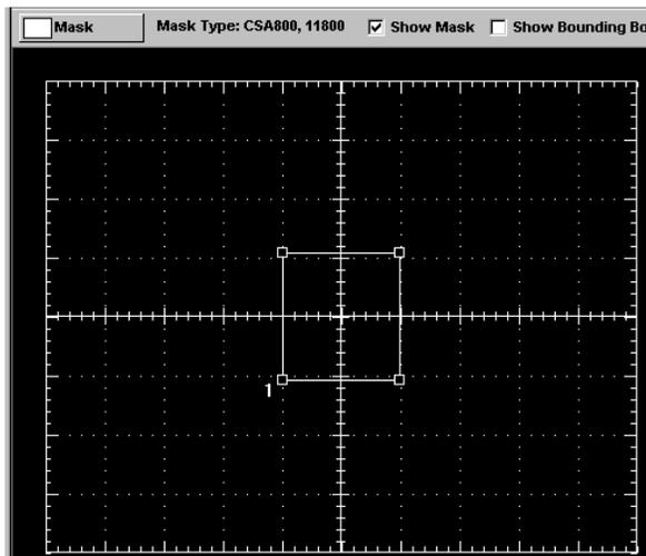
To set the mask parameters, open the Edit Mask Parameters dialog box (**Masks > Tabular View > Edit Parameters...**). The number and type of parameters displayed depends on the parameters supported by the target oscilloscope. Refer to oscilloscope documentation for a description of that instrument's mask parameters.
