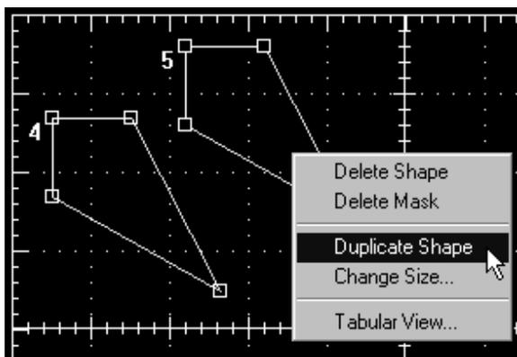
To delete a mask segment, position the cursor within the segment, right-click the mouse, and select **Delete Segment** from the pop-up menu. WaveStar deletes the selected mask segment. You can also delete the entire mask by selecting **Delete Mask** from the pop-up menu.
