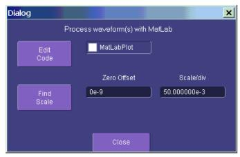
Touch Find Scale to make your output fit the grid, or use the text boxes to choose a scale.
