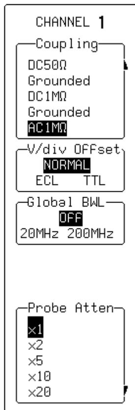
2. Use these menus to set input signal coupling and grounding, the channel bandwidth limit, and the probe attenuation.
