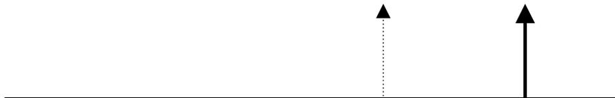
**Figure 8-6. Interval Trigger that triggers when the interval width is smaller than the selected interval. The broken, upward-pointing arrow indicates a potential trigger, while the bold one shows where the actual trigger occurs — on the positive edge within the selected interval.**
