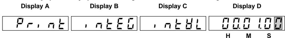
You can change the value at the blinking digit. Pressing the  $\wedge$  key changes the value in the order 1, 2, 3 ... 9, 0 and back to 1. Pressing the  $\vee$  key changes the value in the opposite direction.
