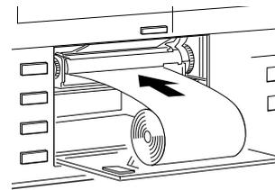
4. Hold down the **FEED** key until approximately 10 cm of the paper comes out of the top of the guide.
