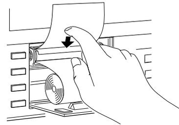
6. Place the paper inside the printer and pass the end of the paper through the slot in the printer cover.
