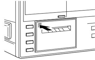
2. Lift the paper feed guide lever in the direction shown by the arrow to release the paper lock.
