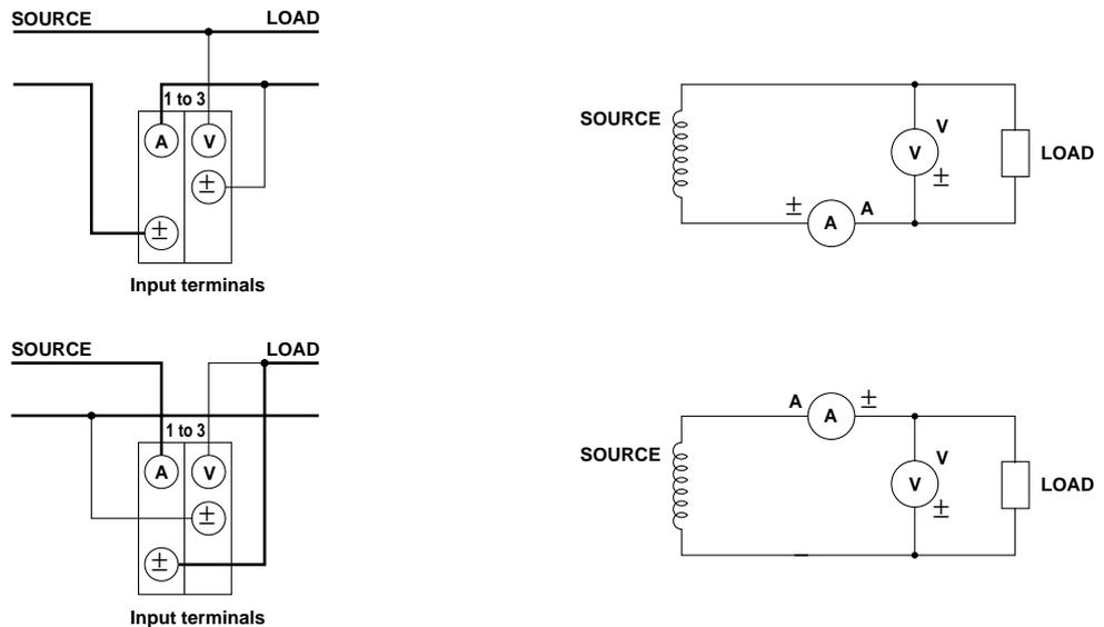
Fig. 3.2 Wiring Diagram for Single-Phase Three-Wire (1Φ3W)
