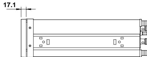
Unless otherwise specified, tolerance is  $\pm 3\%$ . (However, tolerance is  $\pm 0.3$  mm when below 10 mm.)
