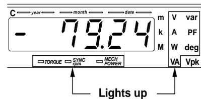
In addition, the torque, synchronous speed and mechanical power obtained using the motor evaluation function (available with the WT1030M only) are also displayed.
