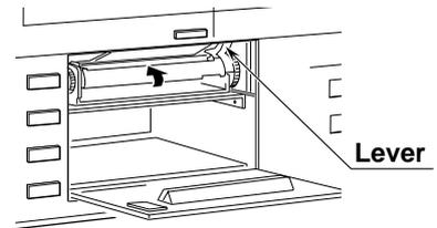
3. Insert the paper underneath the paper feed guide. Make sure that the paper is not skewed. Press the **FEED** key to feed the paper. (Make sure that the paper is fed in the direction as illustrated. If the paper is fed in the opposite direction, printing cannot be performed.)
