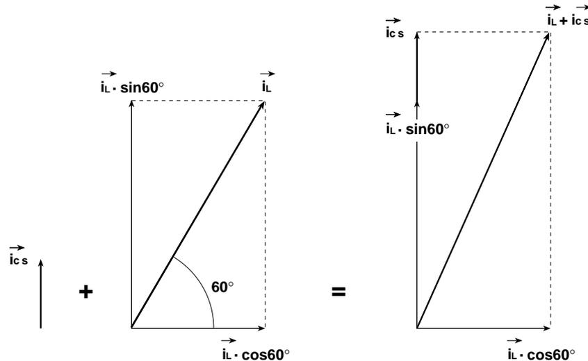
$$\begin{aligned} |\vec{i}_L + \vec{i}_{cs}| &= \sqrt{(i_L \cos 60^\circ)^2 + (i_{cs} + i_L \sin 60^\circ)^2} \\ &= \sqrt{(0.5)^2 + (0.00628 + 0.866)^2} \\ &\cong 1.00542\text{A} \end{aligned}$$
