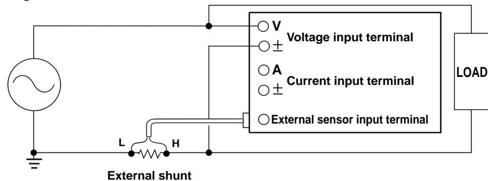
Fig. 3.15 Wiring Example for Single-Phase, Two-Wire (1Φ2W) System with Voltage-Output Type Isolation Sensor (CT, DC-CT, Clamp) Connected
