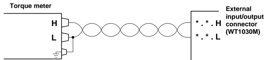
Connect terminal L to the ground at the output side. Make sure that the instrument is also grounded.
