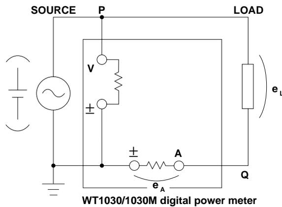
From the above explanation, it can be understood that the effect of instrumental loss on measurement accuracy can be reduced by wiring according to the load resistance.
