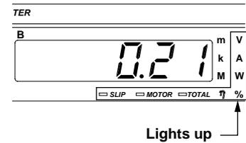
In addition, the slip, motor efficiency and total efficiency obtained using the motor evaluation function (available with the WT1030M only) are also displayed.
