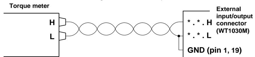
Connect terminal L to the ground pin (1, 19) of the external input/output connector.
