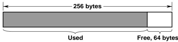
When handshaking is in use, reception of data will stop when the free space in the buffer drops to 64 bytes since data cannot be passed to the main program fast enough to keep up with the transmission.
