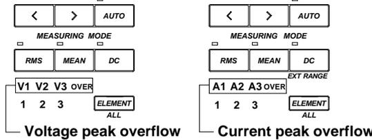
**When measured voltage or current is below 0.5% of the rated value of the range used**
