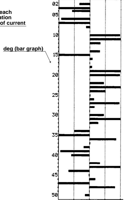
Phase angle of each harmonic in relation of fundamental of current
