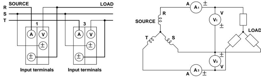
Fig. 3.4 Wiring Diagram for Three-Phase Four-Wire (3 $\Phi$ 4W)
