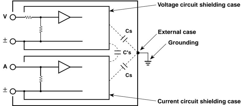
The voltage circuit is enclosed in its own shielding case, and the current circuit is also enclosed in its own shielding case. Both shielding cases are then enclosed in the external case. The voltage circuit shielding case is connected to the  $\pm$  voltage terminal, whilst the current circuit shielding case is connected to the  $\pm$  current terminal.
