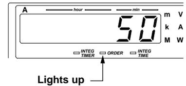
However, due to the fundamental frequency of the PLL source becoming large or from turning the anti-aliasing filter to ON, the Maximum analysis order changes, sometimes resulting in the upper limit of the harmonic order to become larger than the Maximum analysis order. In this case, if the display order is set to a value between the Maximum analysis order and the upper limit of the harmonic order, " - - - - - " will be displayed on display B or C.
