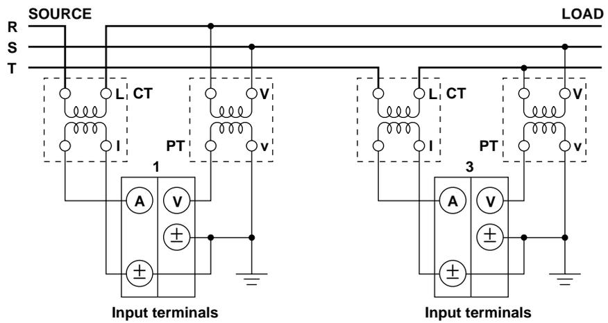
Fig. 3.11 Wiring Example for Three-Phase, Four-Wire (3Φ4W) System with PT and CT Connected
