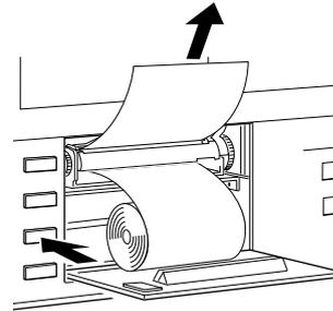
5. Push the middle of the guide in the direction shown by the arrow to secure the paper.
