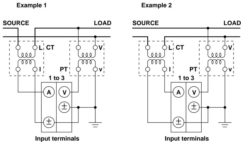
**Fig. 3.9 Wiring Example for Single-Phase, Three-Wire (1Φ3W) System with PT and CT Connected**
