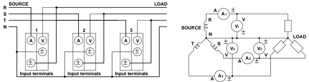
Fig. 3.5 Wiring Diagram for Three-Voltage Three-Current (3V3A)
