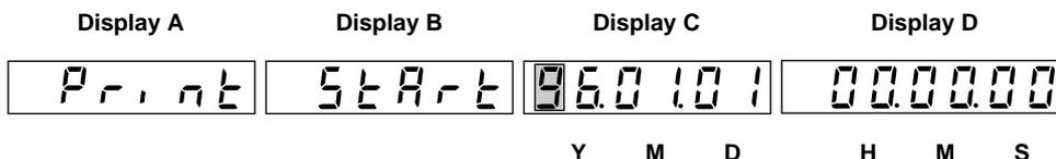
6. The currently selected print output start time will be displayed on display D, with the digit on the extreme left blinking. Set the start time in the same way as step 5.
