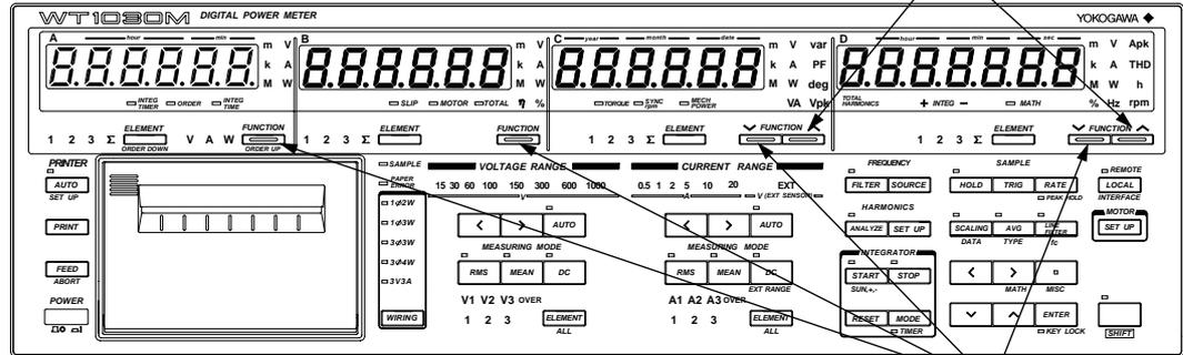
The specific type of information to be displayed is shifted downwards each time the **FUNCTION** key is pressed.
