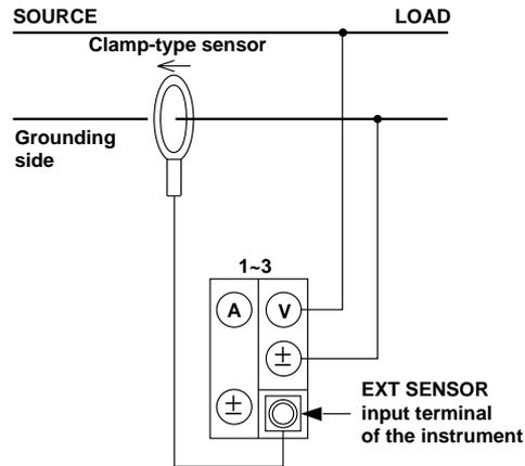
Fig. 3.16 Wiring Example for Single-Phase, Three-Wire (1Φ3W) System or Three-Phase, Three-Wire (3Φ3W) System with Voltage-Output Type Isolation Sensor (CT, DC-CT, Clamp) Connected
