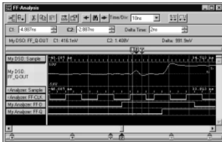
Figure 2-38: Using the DSO module to capture a runt pulse
