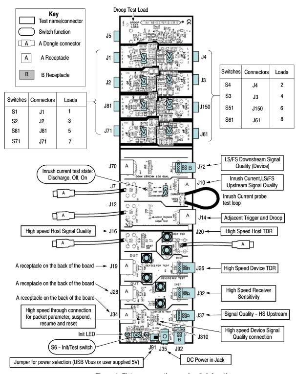
Figure 1: Fixture connections and switch functions
