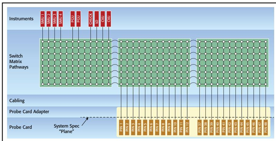
Every S530 system is made up of five layers: instruments, switch pathways, cable interface, probe card adapter, and probe card.
