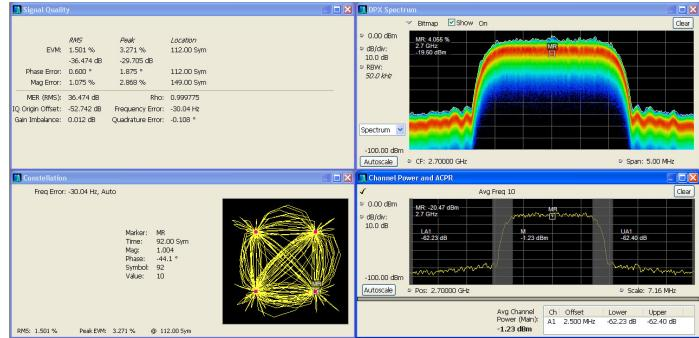
Time-correlated views in multiple domains provide a new level of insight into design problems not possible with conventional analyzers. Here, ACLR and modulation quality are performed simultaneously in a single acquisition, combined with the continuous monitoring of the DPX® spectrum display.
