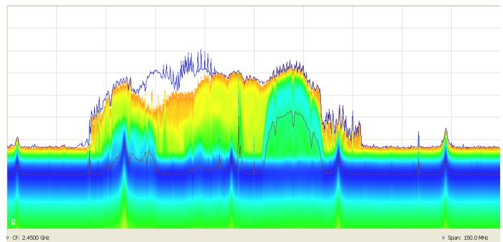
Advanced Triggers, Swept DPX, and Zero Span (Opt. 200) provides superior swept spectrum analysis for transient signals. Here, a 150 MHz swath of spectrum is swept across the ISM band. Multiple WLAN signals are seen, and narrow signals seen in the blue peak-hold trace are Bluetooth access probes. Multiple interfering signals are seen below the analyzers noise level in the multi-color DPX display.
