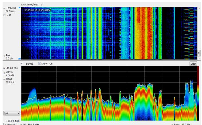
DPX Spectrograms (Opt. 200) provide gap-free spectral monitoring for up to days at a time. 60,000 traces can be recorded and reviewed, with resolution per line adjustable from 110  $\mu$ s to 6400 s.
