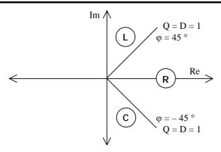
Fig. 6 Definition of the RLC parameters in the complex plane
