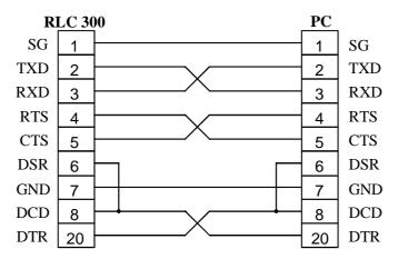
Fig. 2 Plug connections of cable RS-232C
