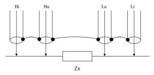
Fig. 3 Connecting the measured object without the adapter
