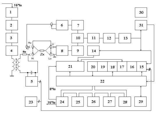
Fig. 1 Block diagram of the RLC 300
