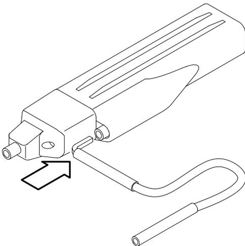
**3- and 6-inch ground leads.** Use the three- and six-inch ground leads for general probing. The socketed end of the leads may be connected to any of the probe tips and adapters, or fitted onto 0.025 inch pins.
