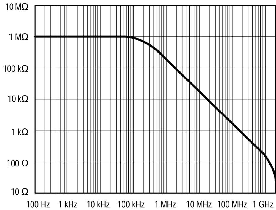
**Figure 3–3: Typical Input Impedance vs. Frequency**
