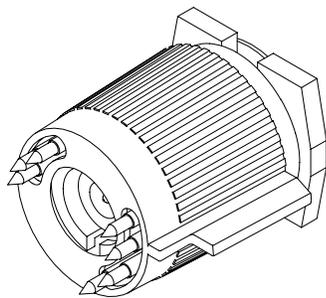
**TEKPROBE Interface.** The TEKPROBE interface provides a communication path between the probe and the oscilloscope. Contact pins provide power, signal, offset, and probe characteristic data transfer. See page 4–2 for more information.
