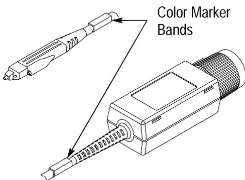
**Color Marker Bands.** Attach matching pairs of the color marker bands onto the cable at the head and compensation box of each probe. The marker bands enable quick verification of which probe is connected to which instrument channel.
