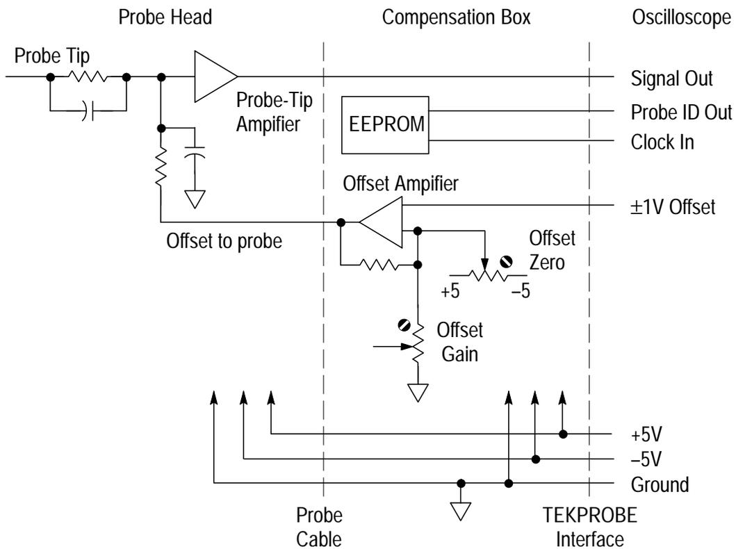
Figure 4–1: P6245AD Simplified Schematic Diagram
