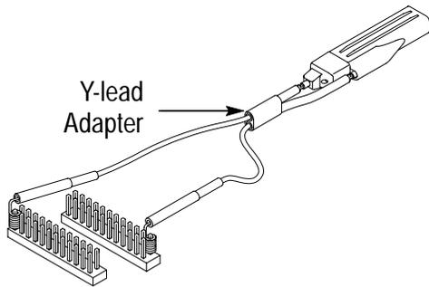
**Y-lead adapter.** Use the Y-lead adapter to extend the physical reach of the probe and ground when necessary. The Y-lead adapter accepts any of the probe tips or adapters, and can be pushed directly onto 0.025 inch pins.
