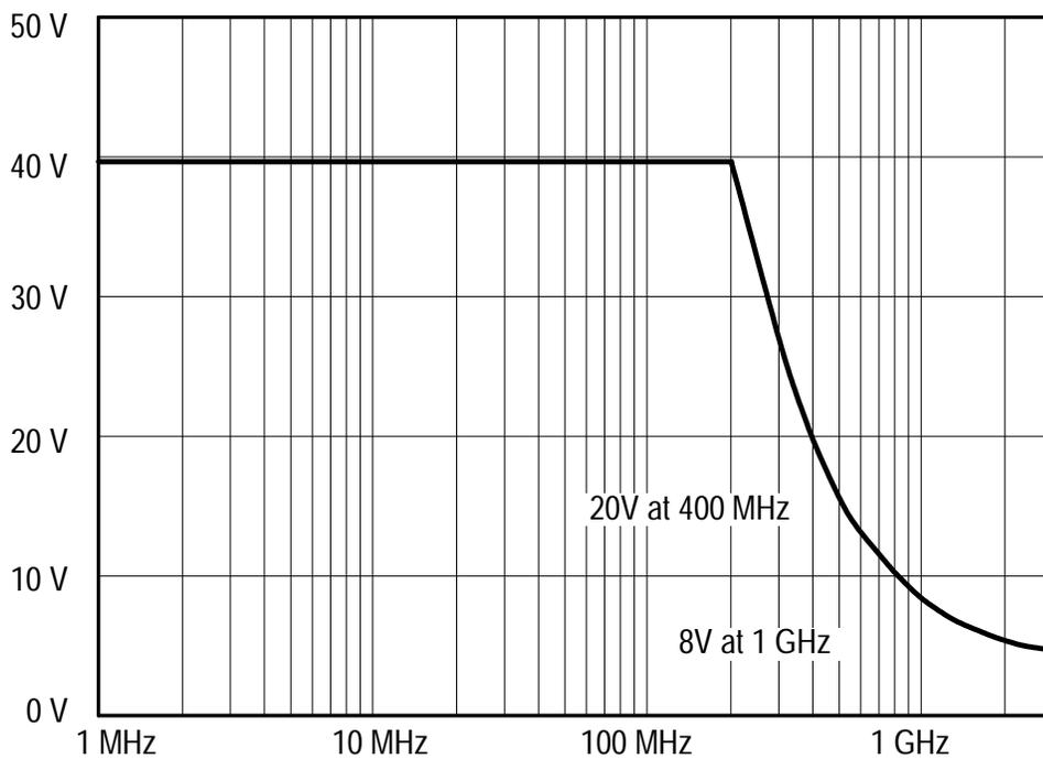
Figure 3-1: Typical Voltage Derating vs. Frequency
