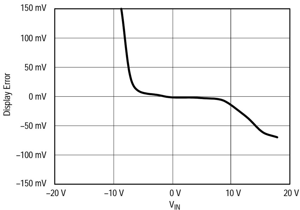
Figure 3-2: Typical Linearity Error vs  $V_{IN}$
