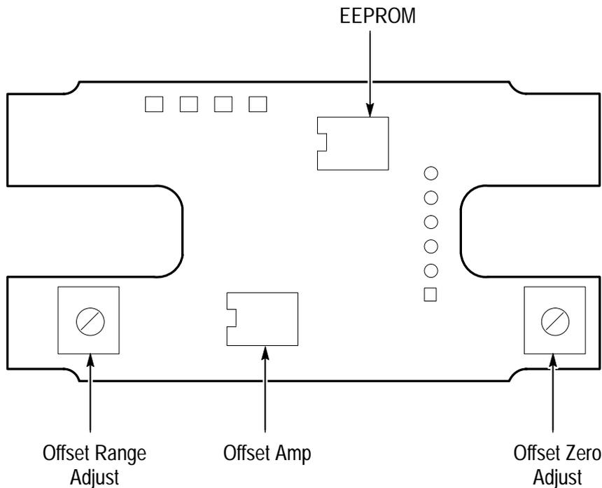
Figure 4-4: P6245AD Adjustment Locations
