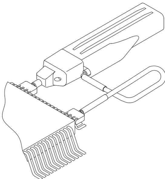
**Figure 2–4: Using a SureFoot Adapter for Grounding**
