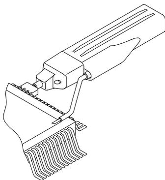
**Low-inductance ground lead.** Use the low-inductance ground adapter to substantially reduce ground lead inductance. Because the ground lead simply touches the ground reference, you can easily move the probe to different points on the device under test.
