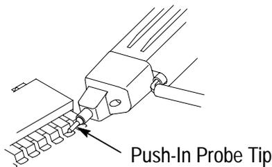
**Push-in Probe Tip.** Use the push-in probe tip for general purpose probing by hand. The tip may also be used as a temporary test point. See page 2–7 for more information.
