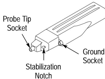
**Probe Head Assembly.** The probe head is designed for ease of use and high performance. Its small size makes it easy to handle in tight areas.
