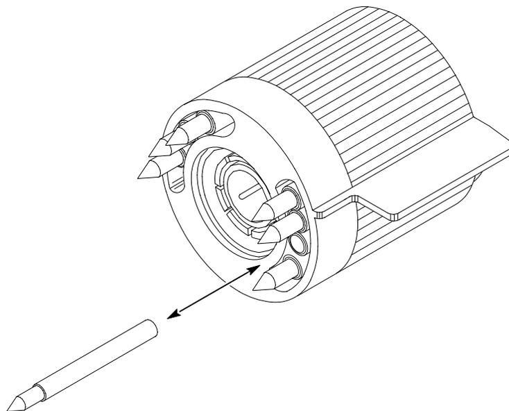
Figure 4–5: Replacing TEKPROBE Interface Pins
