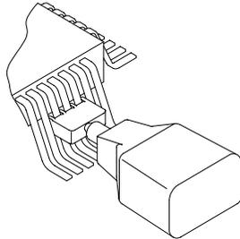
**SureFoot probe tip.** The SureFoot tip is an integral probe tip and miniature guide that enables fault-free probing of fine-pitch SMD packages. Attach the SureFoot adapters the same way as the push-in probe tips. They can be used with any of the socketed accessory leads.
