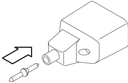
**Installing the Push-in Probe Tip.** Attach the push-in probe tip by seating the tip into the probe tip socket and pushing the tip in until it is seated. Either end of the tip may be used. *Do not force the tip.* Also, be careful not to poke yourself with the sharp probe-tip. To remove the tip, *gently* grab the tip with small pliers and pull the tip out.
