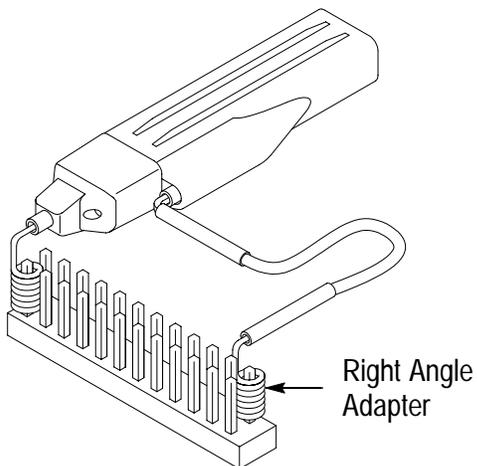
**Right-angle adapter.** Use the right-angle adapter for low-profile probing of 0.025 inch diameter square pins.
