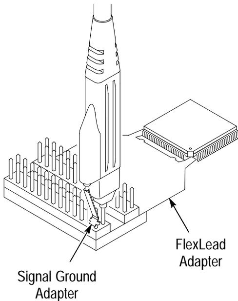
**Signal-Ground Adapter.** The signal-ground adapter is ideal for use with signal/ground pairs on 0.100 inch header pins (such as FlexLead adapters).
