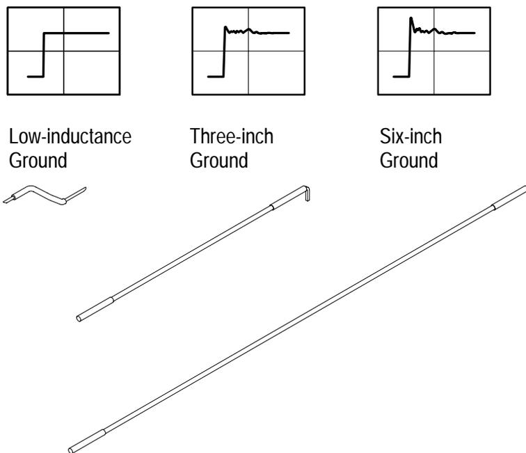
**Figure 2–1: Waveform Distortion from Ground Lead Length**
