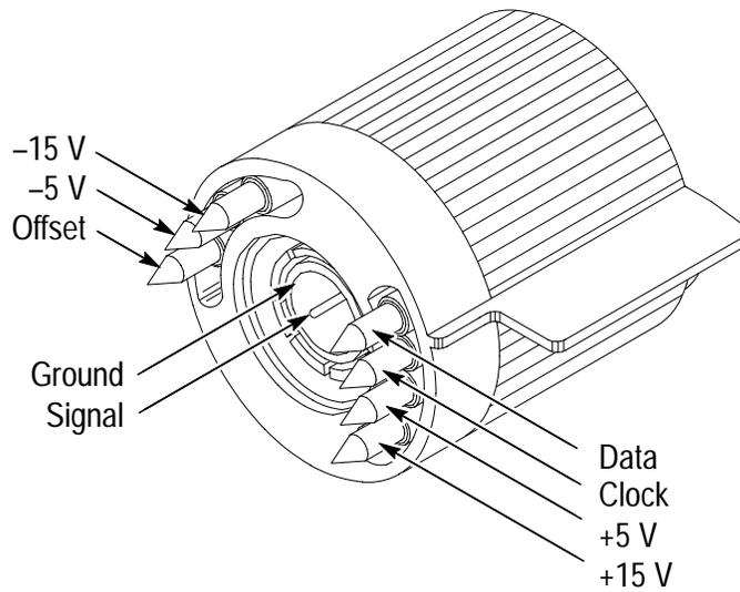
Figure 4–2: TEKPROBE Interface
