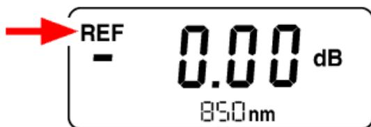
Fig. 4-7 Storing a reference level
