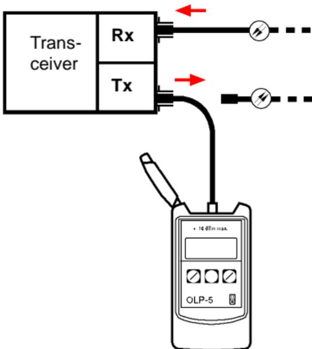
Fig. 4-2 System power level measurement
