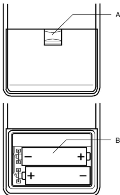
Fig. 3-4 OLP battery compartment, rear of device
