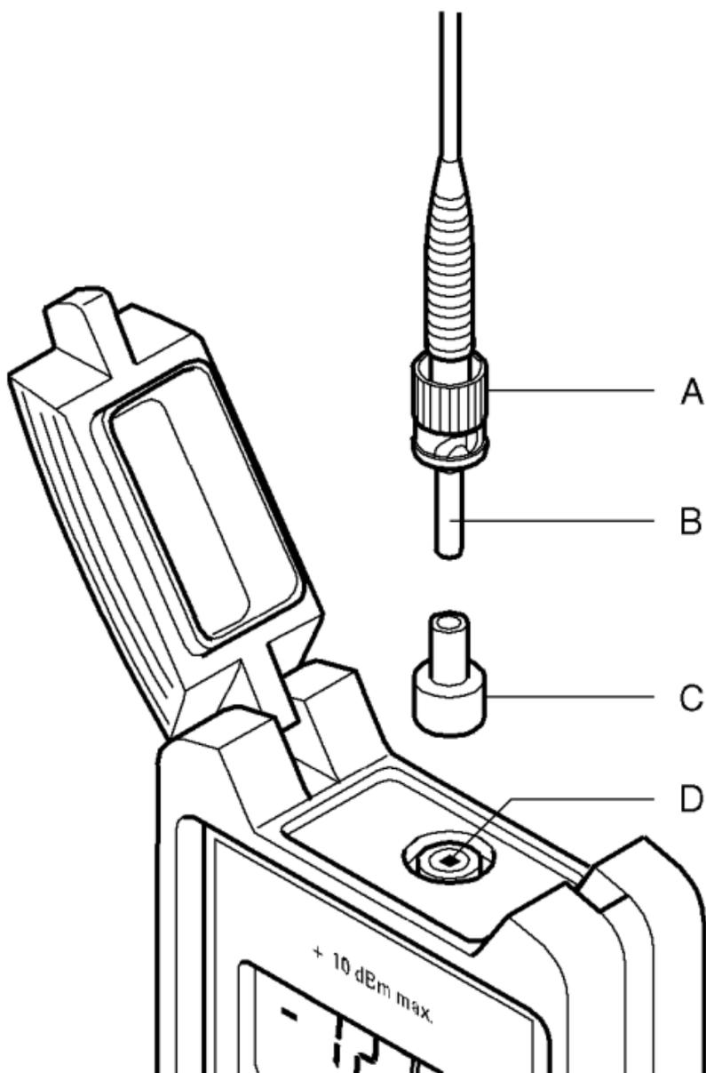
Fig. 3-5 OLP test port with universal adapter
