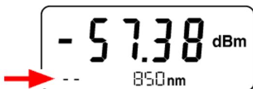
Fig. 4-9 Modulation frequency field for very low levels
