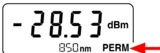
Fig. 3-7 The device is now ready to go! It is in permanent operating mode, and the “PERM” indicator appears.
