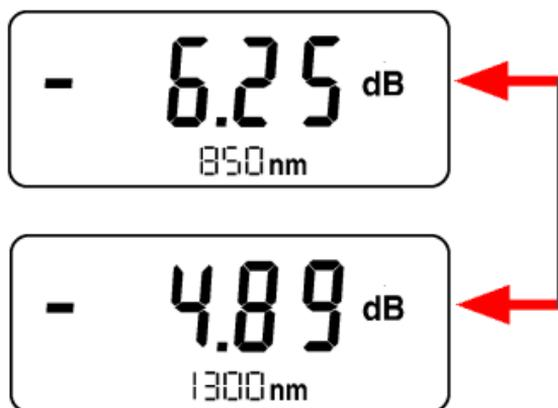
Fig. 4-10 Attenuation display in TWINtest mode
