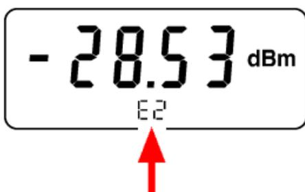
Fig. 5-1 Error message in LC display, e.g. "E2"
