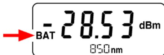
Fig. 3-2 *BAT* indicator with low batteries
