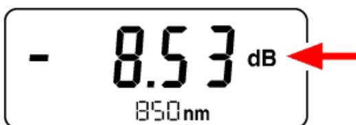
Fig. 4-6 Relative power level display in dB
