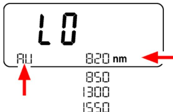
Fig. 4-4 Setting the wavelength, e.g. with the OLP-5; “AU” means automatic wavelength detection is activated
