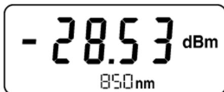
Fig. 3-6 The device is ready to operate as soon as a measured value is displayed along with the other indicators.
