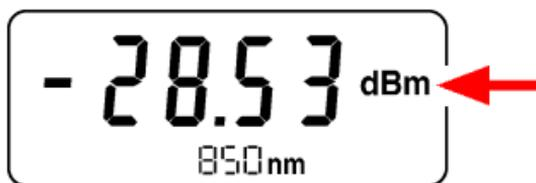
Fig. 4-5 Absolute power level display in dBm. Evaluation of unmodulated light (the modulation frequency field is empty)
