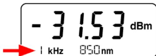
Fig. 4-8 Measuring modulated light. An indicator appears in the modulation frequency field.
