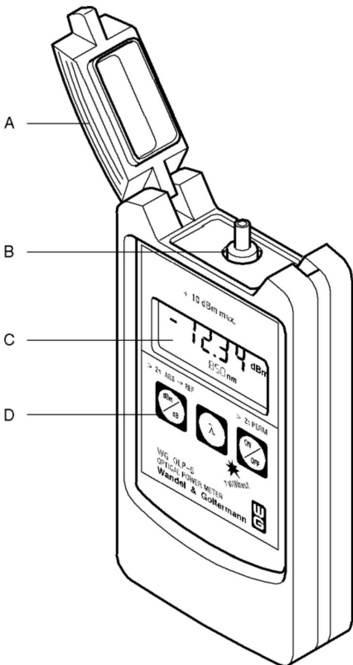
Fig. 4-1 OLP front-panel view with controls and display elements
