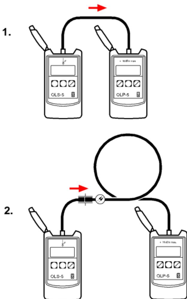
Fig. 4-3 Two-step attenuation measurement
