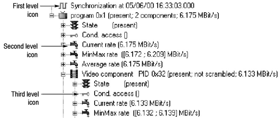
**Figure 3-17: Hierarchy levels in the Analysis Results area**
