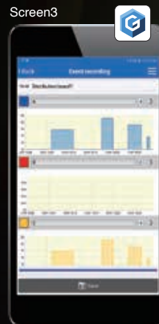
Visualize intermittent GFCI and RCD trips Review trip times and maximum current values
