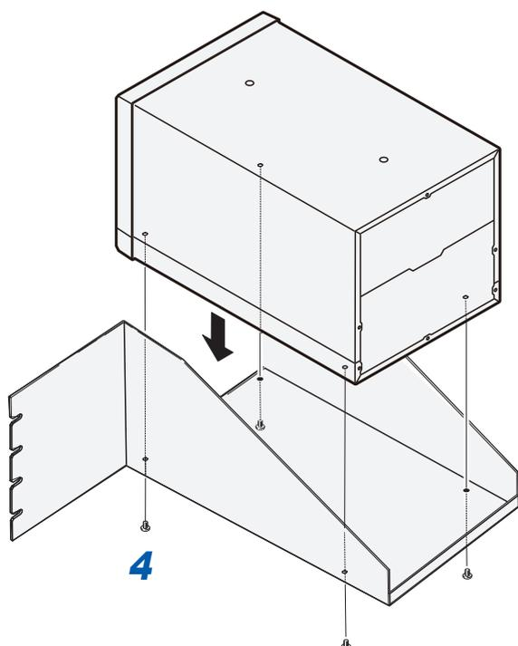
**4** Mount the instrument to the rack metal fittings, and secure from the bottom using countersunk screws (M3 × 10 mm) ×4.
