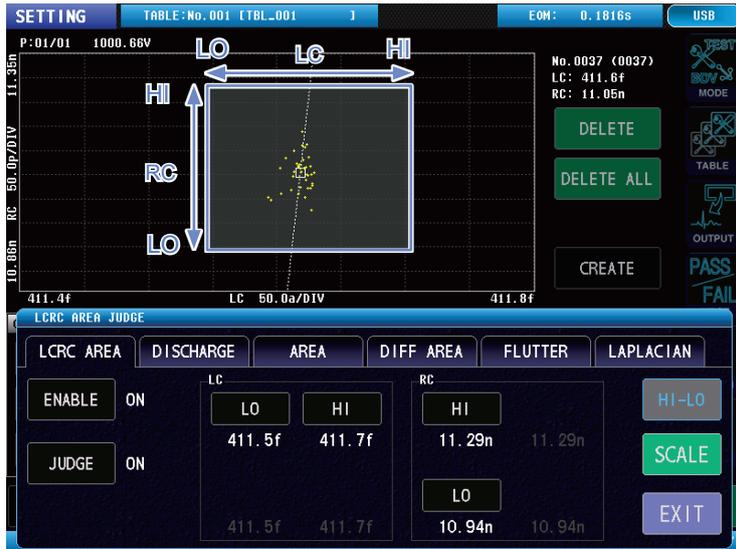
**[HI-LO] is OFF (Threshold value set using LC and RC values zeniths)**
