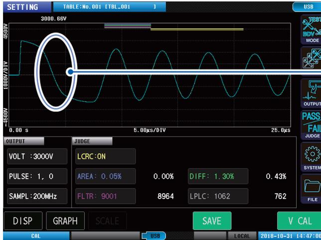
If the core is magnetically saturated, the waveform will tilt rapidly.
