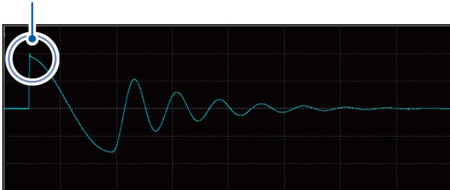
Even if the response waveform max. peak voltage is outside the primary peak, adjust so that the max. peak voltage value is the same as the set voltage value.
