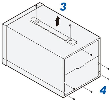
**3** Remove the screws ×2 that secure the handle on the top, and remove the handle.
