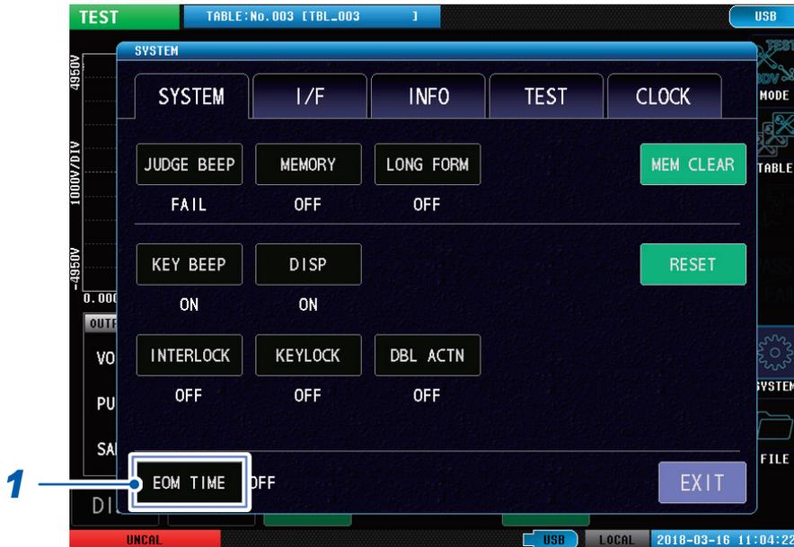
1 Tap [EOM TIME], and set whether to display or hide the test times (EOM).
