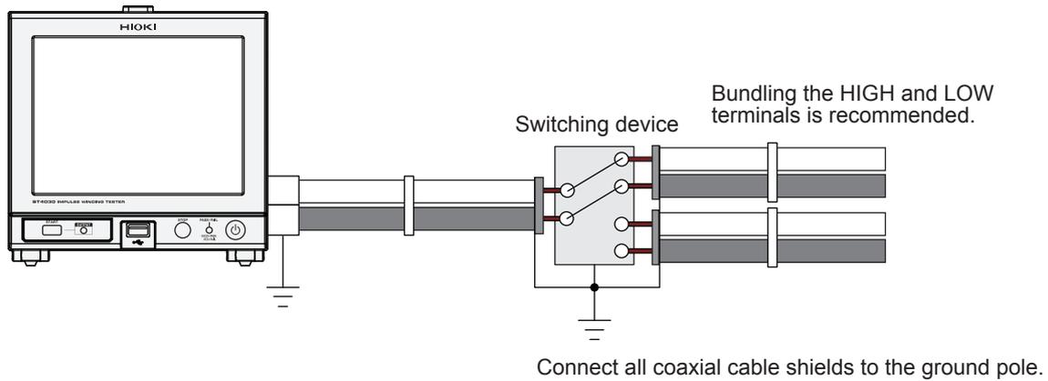
In the case of the diagram below, the cable shields are connected via the case of the switching device to comprise the instrument ground pole. A shorter distance for the core switching unit is recommended.
