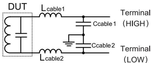
The inductance of the 2 cables enters the workpiece to be tested serially.
