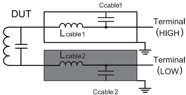
There is parasitic capacity between the core of the coaxial cable and the shield ( $C_{\text{cable1}}$ ,  $C_{\text{cable2}}$ ). Model L2250 capacity is approx. 180 pF each.
