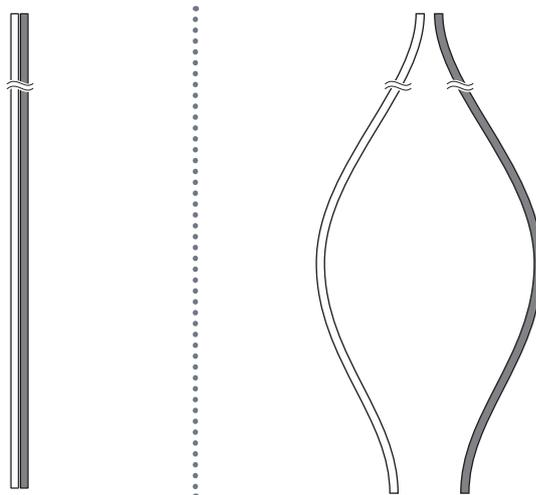
Variations in oscillation frequency and variations in measurement cable inductance will have a particularly significant effect on test results when testing low-inductance workpieces. It is recommended that you bundle the 2 cables as shown below to minimize impedance changes due to shape.
