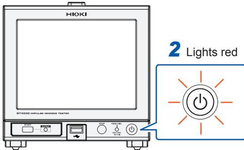
**1** Turn ON the main power supply switch with the power cord connected.
