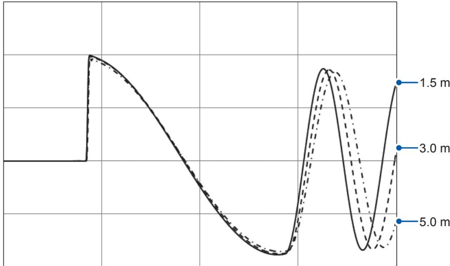
Using a longer test lead increases the cable capacity (C). According to  $T=2\pi\sqrt{LC}$ , the longer the lead, the longer the oscillation period.
