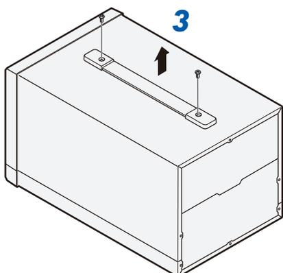
**3** Remove the top screws ×2, and remove the handle.
