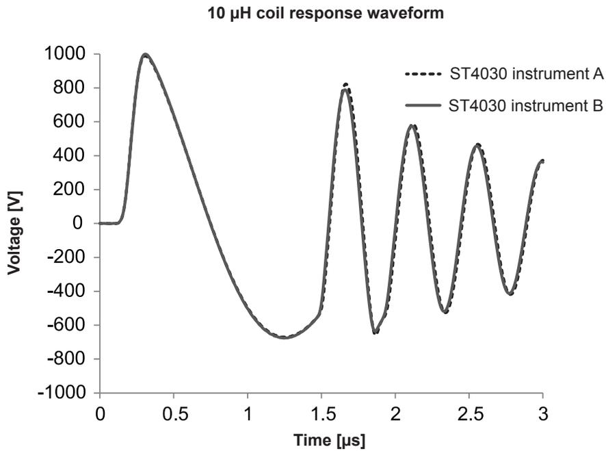
When switching instruments, either set with sufficient space to that the judgment threshold values are not affected by the instrument differences, or recalibrate the voltages and then reset the judgment threshold values.
