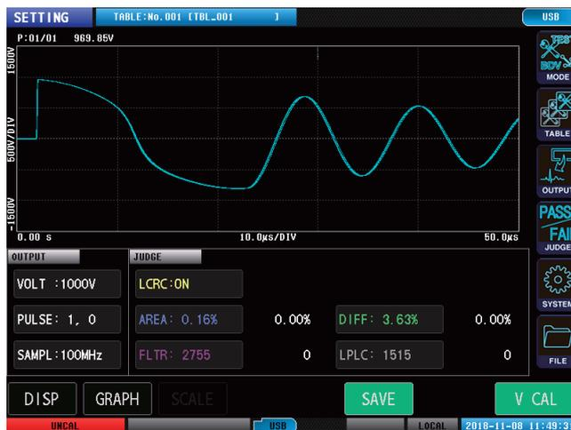
You can see how waveforms diverge by turning on waveform superposition and repeating the test multiple times.
