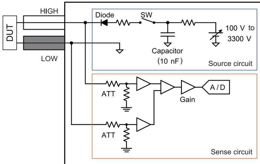
The circuit operations after testing starts are as described below.
