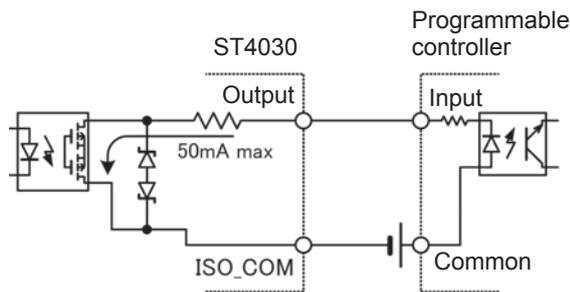
Connection to programmable controller (positive common inputs)
