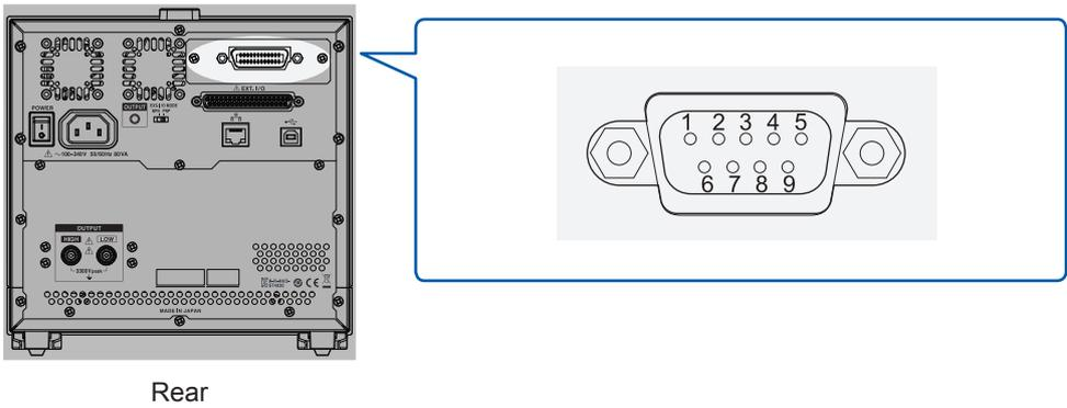
When connecting a controller (DTE), prepare a instrument connector and a cross cable with the controller connector specifications.
