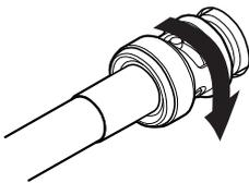
When removing, rotate the coaxial connector on the connection cable to the left and then pull out.
