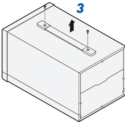
**3** Remove the top screws ×2, and remove the handle.
