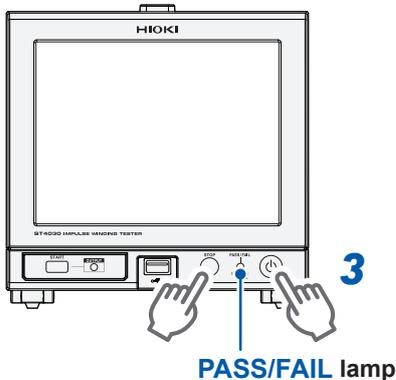
**3** Press and hold the **STOP** button, and press the start button.
