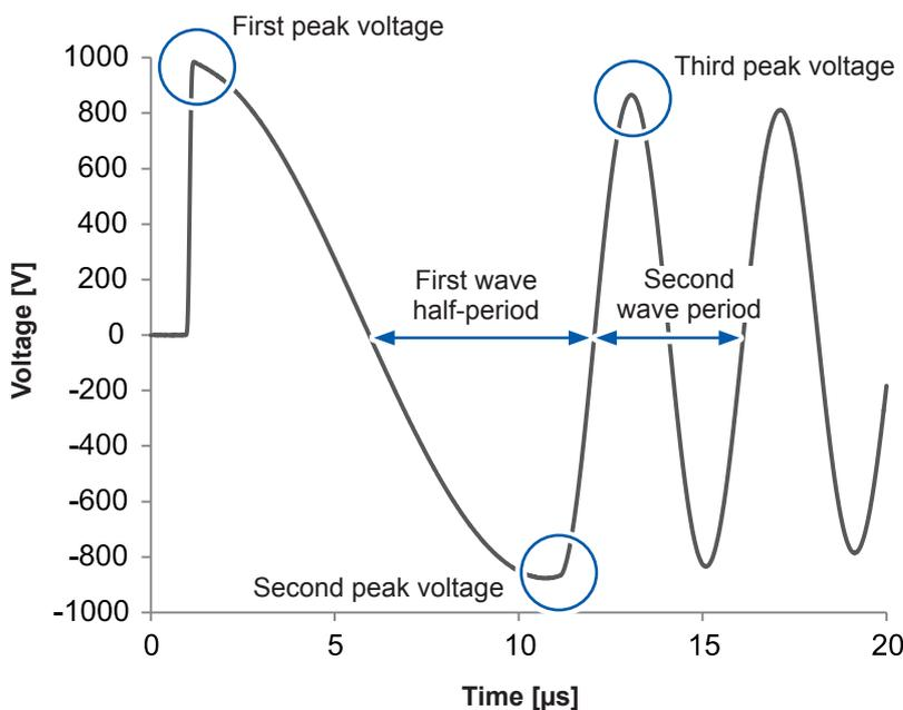
Describes the instrument differences determined using the waveforms obtained using each Model ST4030.
