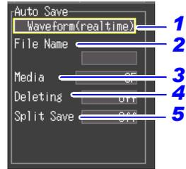
Horizontal axis settings are inhibited during automatic saving of waveforms (p. 49).
