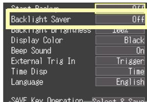
Be aware that power is still consumed even when the backlight is off, so be sure to turn the instrument's power switch off when not in use.
