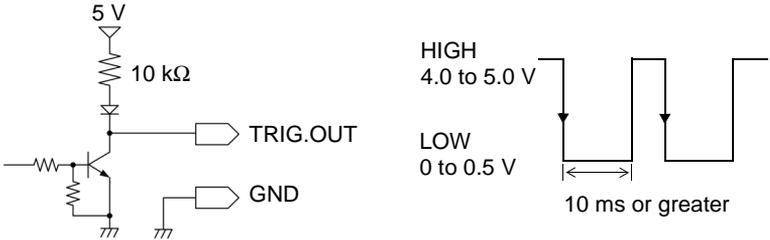
**NOTE** When triggering is not otherwise used, a trigger signal is output during measurement.
