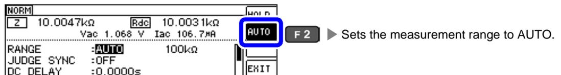
Outside the accuracy guarantee range, AUTO ranging may not function properly, preventing a range from being selected. If this occurs, check the accuracy guarantee range in "11.2 Measurement Range and Accuracy" (p.204) and change the measurement conditions.
