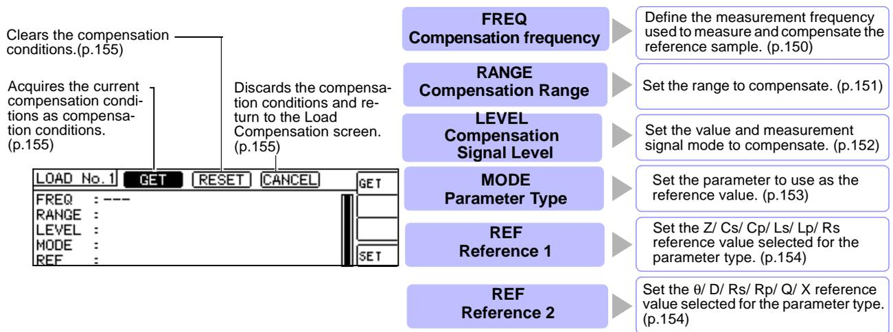
The compensation coefficient is computed from the reference values of Z and θ obtained from the set values and the actual data acquired from the reference sample at each of the compensation frequencies.
