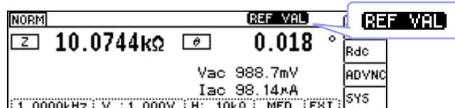
If the measurement value is outside the accuracy guarantee, **REF VAL** will be displayed at the top of the screen. Check the accuracy guarantee range in "11.2 Measurement Range and Accuracy" (p.204) and either change the measurement conditions or make the measurement value a reference value.
