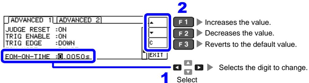
**NOTE** The output time cannot be set unless the output method is set to pulse.
