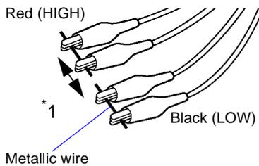
Short the probe's Hcur and Hpot terminals (red) with one metallic wire and its Lcur and Lpot terminals (black) with the other, so that there is no connection between the high and low terminals. Perform open correction.
