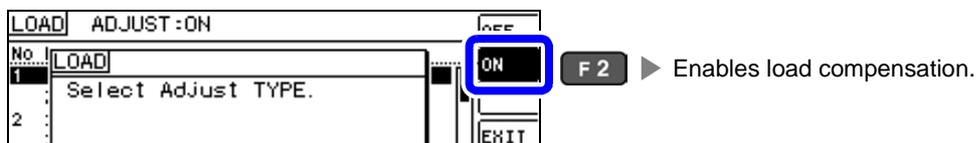
6.3 Adjusting Values Based on Reference Values(Load Compensation)
