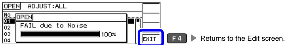
The open circuit compensation process is quite sensitive to noise - both noise originating externally and induced noise. Therefore, if open circuit compensation has been interrupted with a fault, you should check the following points before starting the compensation process again (p.125):
