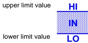
Set absolute values for the upper limit and lower limit values of the measurement parameters.
