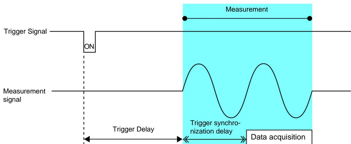
**NOTE** When the range synchronization function has been set, the range settings at which the trigger delay and trigger synchronous output function are enabled vary with the parameter settings.
