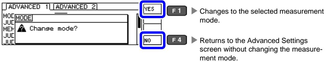
**4** The measurement mode will be changed to continuous measurement mode.
