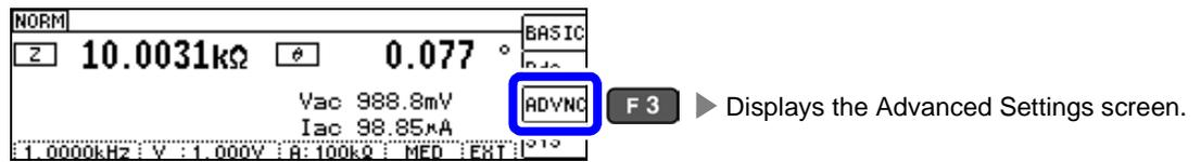
**2** Set the Hi Z reject function to [OFF] or [ON].
