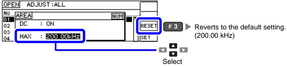
7 Enter the desired value with the tenkey and accept it with the **ENTER** key. **10KEY**
