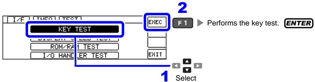
**4** Press the rubber keys to perform the key test. Verify that the key on the screen corresponding to the key you pressed is shown in reverse video.
