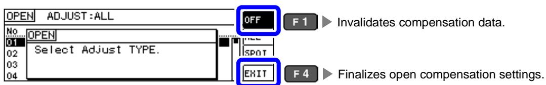
**NOTE** The compensation values that are stored internally are not cleared by the operation described above. When ALL or SPOT is selected, the stored compensation values can be used.
