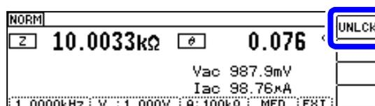
F1 ► Select [UNLCK] on the Key Lock screen. Displays the Passcode Entry screen.
