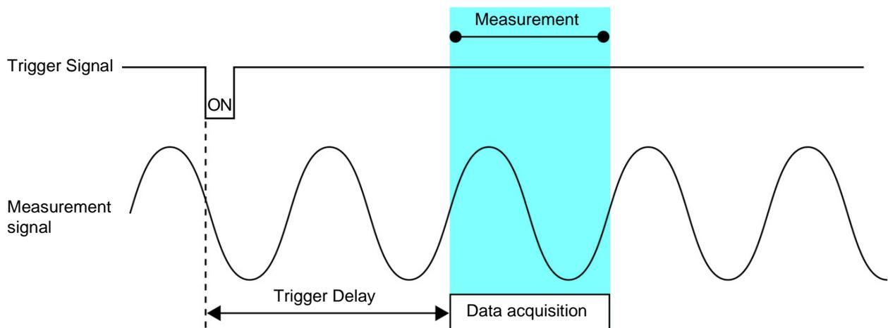
Trigger delay: ON; Trigger synchronous output: ON
