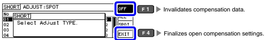
**NOTE** Performing the operation described above will not delete compensation values stored in the instrument's memory. The saved compensation values will be used when ALL or SPOT is selected.
