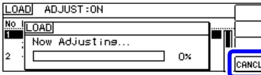
F 4 ▶ Cancels the load compensation operation and returns to the Compensation screen. (The previous load compensation values will be used.)
