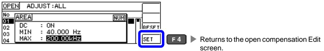
**NOTE** If the maximum compensation frequency is less than the minimum compensation frequency, the minimum and maximum compensation frequencies will be switched automatically.
