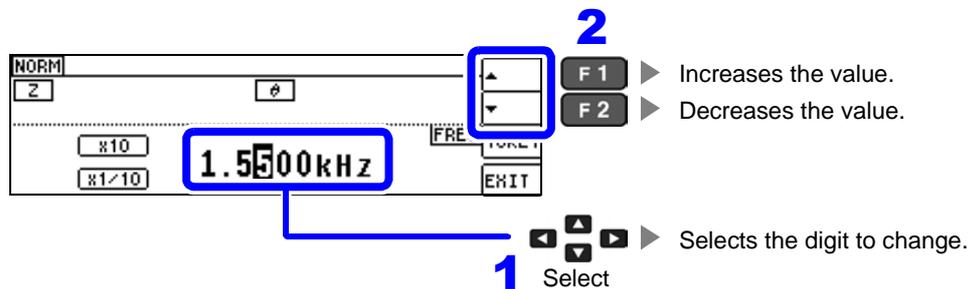
**NOTE** The digits in the measurement frequency can also be changed using the ▲ ▼ keys.
