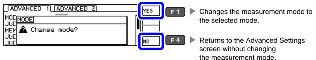
**NOTE** After changing the measurement mode, check all settings (including compensation) before performing measurement.
