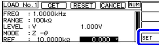
F 4 ▶ Accepts the compensation conditions and returns to the load compensation Edit screen.
