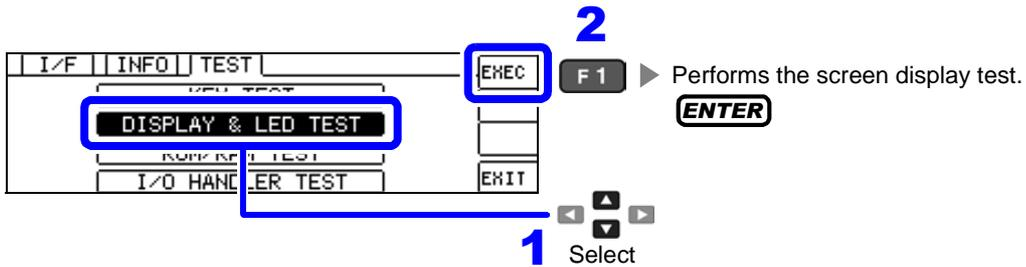
Each time you press **ENTER**, the screen and the LEDs on the front of the instrument will cycle on and off in the following order:
