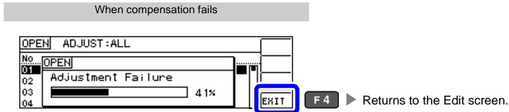
The open circuit compensation process is quite sensitive to noise - both noise originating externally and induced noise. Therefore, if open circuit compensation has been interrupted with a fault, you should check the following points before starting the compensation process again (p.125):
