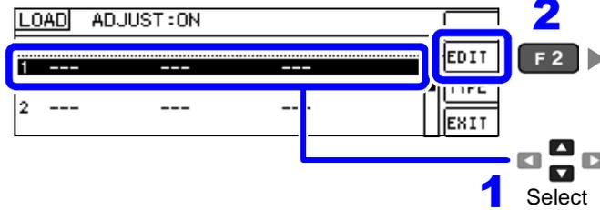
F 2 ▶ Displays the load compensation conditions Edit screen.
