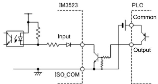
PLC Input (Source Input) Connections
