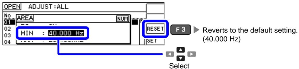
**5** Enter the desired value with the tenkey and accept it with the **ENTER** key. **10KEY**
