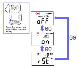
To exit sub-function mode, press the power key to turn off the instrument and then turn it back on
