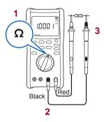
The open terminal voltage is approx. 2.5 V or less. The measurement current (DC) varies depending on the range. (p. 86) To avoid damage to the measurement object, check the specifications before use.
