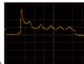
Starting current in a car starter 100A/div, 1s/div
