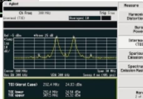
TOI – Easily quantify distortion performance. With the automated third order intercept measurement, you can conveniently quantify the intermodulation immunity of your device.
