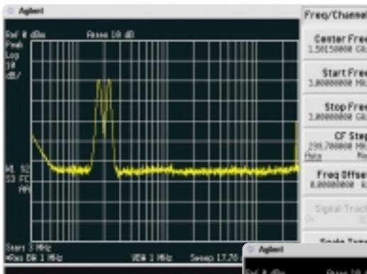
When using it for applications like the testing of switching power supplies, a log sweep will expand the lower end of the band giving you a closer look at the individual signals in that frequency range while still maintaining a wide analyzer frequency span.
