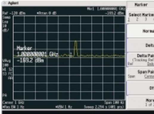
The ESA-E Series has digital narrow resolution bandwidth filters and internal preamplifiers so you can identify low-level spurs.
