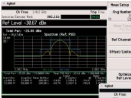
Quickly determine the in-channel power and out-of-channel power spurious emissions as required for W-CDMA and wireless LAN formats. Flexibility in the spectrum emission mask (SEM) measurement allows you to select up to five offsets with individual settings for RBWs and limits.
