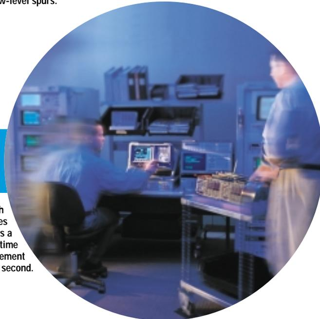
For circuit adjustments with real-time results, the ESA-E Series spectrum analyzers offers a one-millisecond sweep time and up to 45 measurement updates per second.
