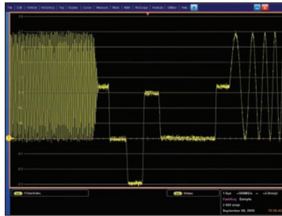
Triggering on an analog HDTV tri-level sync signal and examining horizontal blanking interval.
