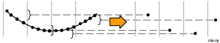
**Envelope** mode finds the highest and lowest record points over all acquisitions. Envelope uses Peak Detect for each individual acquisition.
