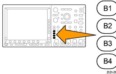
2. Turn multipurpose knob **a** to adjust the vertical position of the selected bus.
