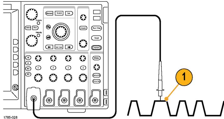
2. Select the input channel by pushing the front-panel buttons.
