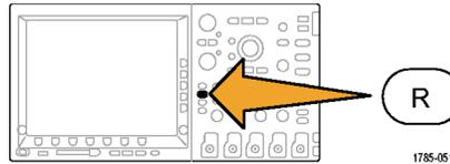
2. Use the resulting lower-bezel menu selections to display or select a reference waveform.
