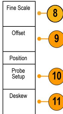
9. Select **Offset** to enable multipurpose knob **a** to make vertical offset adjustments.
