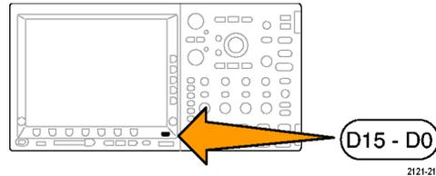
6. Push the lower-bezel **D15 - D0** button to access the D15 - D0 On or Off menu.
