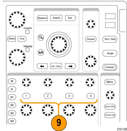
10. **B1** or **B2**. Push to define and display a bus if you have the appropriate module application keys. The DPO4AUTO module supports CAN and LIN buses. The DPO4AUTOMAX supports CAN, LIN and FlexRay buses. The DPO4EMBD module supports I<sup>2</sup>C and SPI. The DPO4COMP module supports RS-232, RS-422, RS-485, and UART buses.
