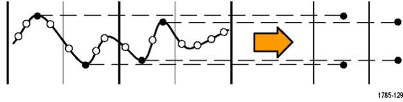
**Hi Res** mode calculates the average of all the samples for each acquisition interval. This mode also only works with real-time, noninterpolated sampling. Hi-Res provides a higher-resolution, lower-bandwidth waveform.
