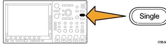
Now you want to measure the width of each displayed pulse. You can use measurement gating to select a specific pulse to measure. To measure the second pulse:
