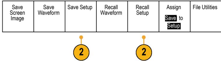
3. From the resulting side-bezel menu, select the location to save the setup to or to recall it from.
