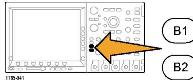
2. Push a lower-bezel button to create a label, such as for channel 1 or B1.
