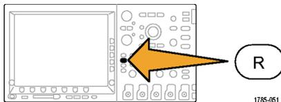
2. Push the **R1**, **R2**, **R3**, or **R4** lower-bezel button to remove the reference waveform from the display.
