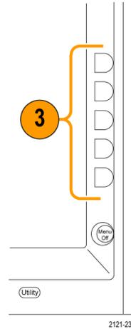
4. To remove a side-bezel menu, push the lower-bezel button again or push **Menu Off**.
