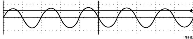
1. Turn the front-panel Trigger **Level** knob to adjust the trigger level without going to a menu.
