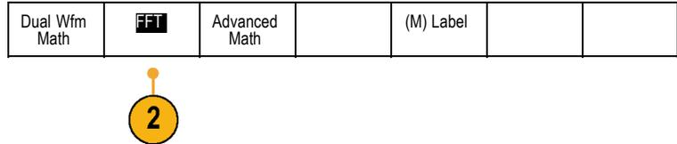
3. Push the side-bezel menu **FFT Source** button, if needed, and turn multipurpose knob **a** to select the source to use. Choices are: channels 1, 2, 3, 4, reference waveforms 1, 2, 3, and 4.
