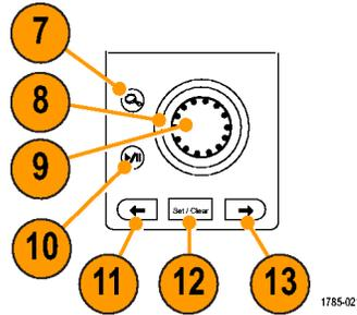
12. **Set/Clear Mark.** Push to establish or delete a waveform mark.
