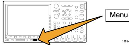
2. Push **Save Setup** or **Recall Setup** from the lower-bezel menu.
