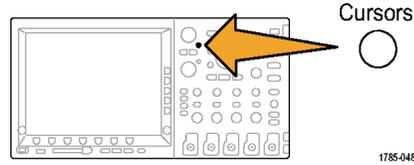
6. Place one cursor on the first peak of the ring using multipurpose knob **a**.
