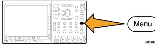
6. Push **Type** to select **Bus**. Enter trigger parameters in the resulting screen menus.
