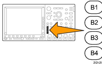
6. Push the **Bus Display** lower-bezel button, push the **Bus and Waveforms** side-bezel button, and push the **ASCII** side-bezel.
