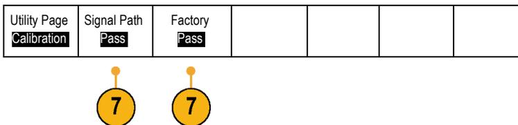
8. Service personnel use the factory calibration functions to calibrate the internal voltage references of the oscilloscope using external sources. Refer to your Tektronix field office or representative for assistance with factory calibration.
