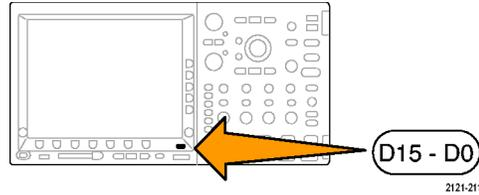
4. Push the **D15-D0 On/Off** lower-bezel button and then push the **Turn On D7-D0** side-bezel button to display the digital waveforms. To turn off a channel, use multipurpose knob **a** to select the channel and push the **Display** side-bezel button to select Off.
