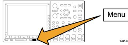
2. Push **Save Waveform** or **Recall Waveform** from the lower-bezel menu.
