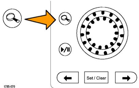
3. Examine the zoomed view of the waveform that appears on the larger, lower portion of the display. The upper portion of the display will show the position and size of the zoomed portion in the waveform, within the context of the overall record.
