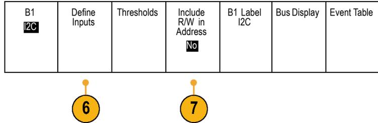
7. For **I2C**, push **Include R/W in Address** and then push the desired side-bezel button for Yes or No. This control determines how the oscilloscope shows the I2C addresses in bus decode traces, cursor readouts, Event Table listings, and trigger settings.
