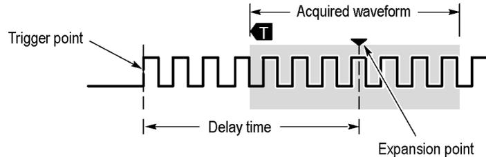
With **Delay** set to **On**, turn the **Horizontal Position** knob counterclockwise to increase the delay. The trigger point will move to the left and ultimately outside of the acquired waveform. Then you can adjust the **Horizontal Scale** knob to acquire more detail around the area of interest at the center of the screen.
