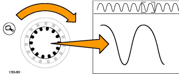
2. Turn the **Pan** knob to place the center of the zoom box close to where the relay contact begins to open.
