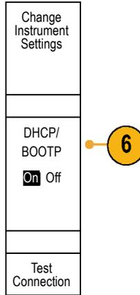
**NOTE.** Depending on the type and speed of network to which your 4000 series oscilloscope is connected, you may not see the DHCP/BOOTP field update instantaneously after pressing the DHCP/BOOTP button. It may take a few seconds to update.
