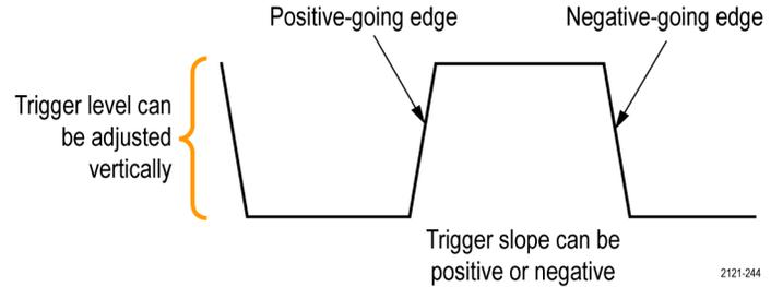
The oscilloscope provides a long horizontal bar or bars across the graticule to temporarily show the trigger level.
