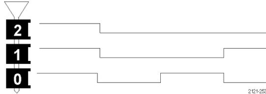
18. The bus display shows decoded packet level information for serial buses or for parallel buses (MSO4000 series only). The bus indicator shows the bus number and bus type.
