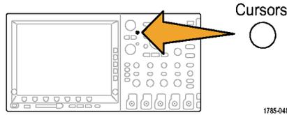
6. Turn multipurpose knobs **a** and **b** to move the pair of horizontal cursors.
