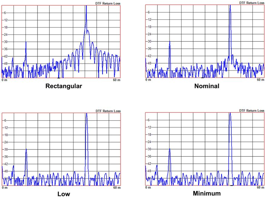
**Figure 3-11.** Effects of Windowing on a Sample Trace
