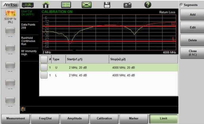
Figure 3-24. Table of Limit Lines (or Segments)
