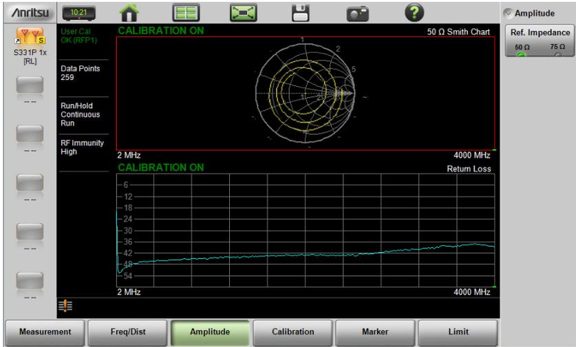
Figure 3-45. Set Reference Impedance for Smith Chart Measurement
