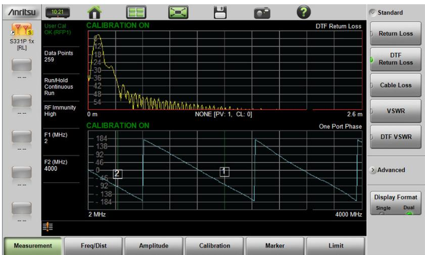
**Figure 2-10.** Dual Display Format with Top Display Active
