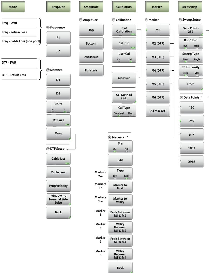
Figure 4-2. Cable & Antenna Analyzer Classic Mode Menu Map
