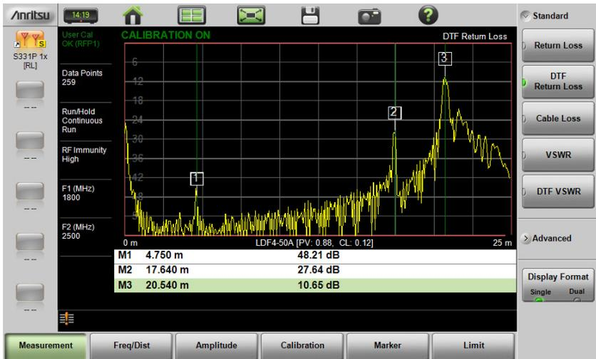
Figure 3-16. DTF Return Loss Measurement (Antenna at 20.54 m)
