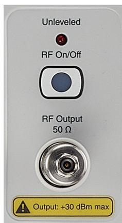
**Unleveled Indicator:** The unleveled indicator is displayed when the RF output goes unleveled and is normally caused by exceeding the specified leveled power rating.
