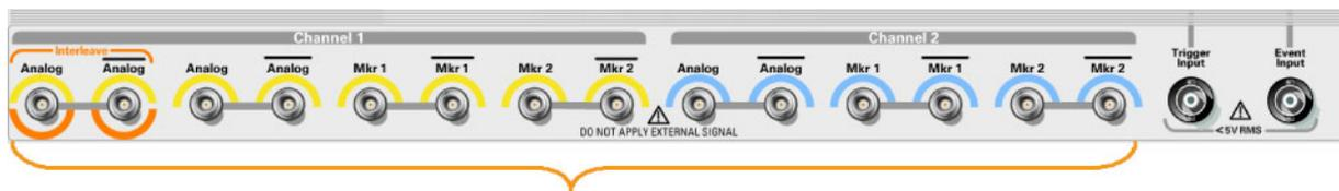
To prevent damage to the instrument, do not apply external voltages to the output connectors.
