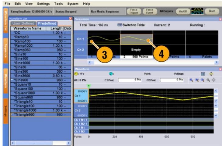
5. Create a sine waveform with the following attributes and set the waveform to the third cell of Ch 1 sequence.
