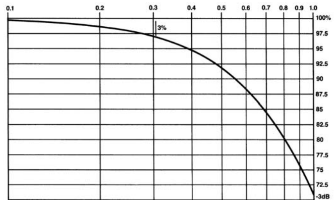
Figure 4.8. Bandwidth derating curve.
