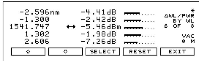
To determine channel spacing, simply read the relative wavelength measurement of the laser lines immediately preceding and following the reference. Use the  $\leftarrow$ ,  $\rightarrow$ , and *SELECT* softkeys to change the reference laser line and read the channel spacing between each channel.
