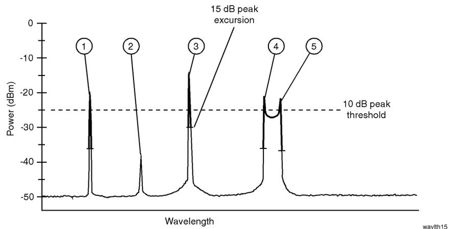
The following figure shows the same laser lines as the previous figure, but the peak-excursion value has been changed from 15 to 3 dB. Four laser lines are now identified with responses  $\emptyset$  and  $f$  identified as two distinct laser lines.
