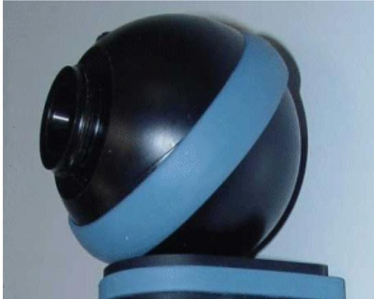
Figure 4 Attaching the Rubber Ring
