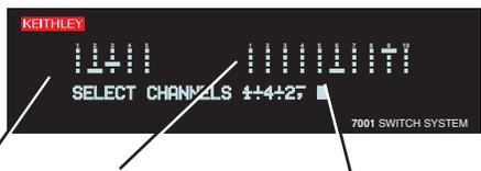
Multiplexer card display. The first row across represents channels 1 to 10. The second row is channels 11 to 20. Only the available channels are displayed.
