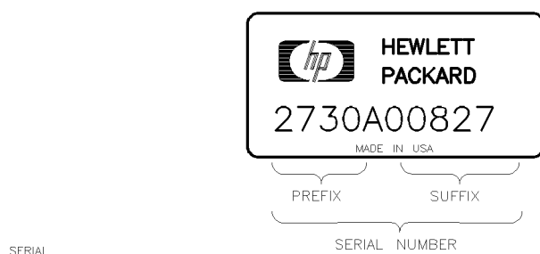
Figure 2-8. Typical Serial Number Label
