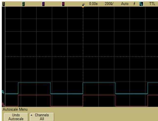
**Figure 7** Autoscale of digital channels 0 & 1 (MSO models only)
