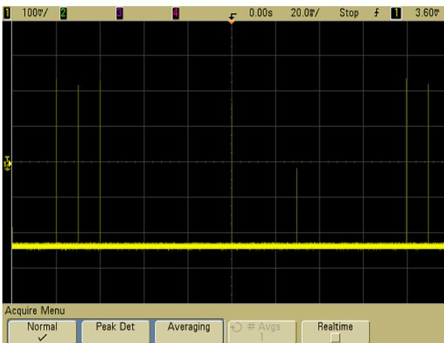
**Figure 41** 15 ns Narrow Pulse, 20 ms/div, Normal Mode
