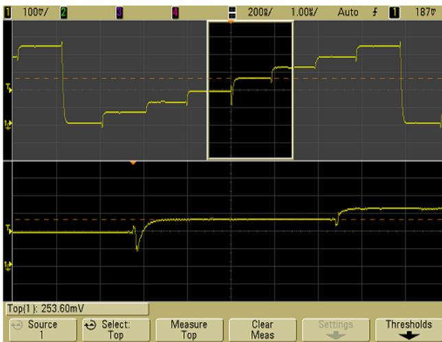
**Figure 35** Isolating area for Top measurement
