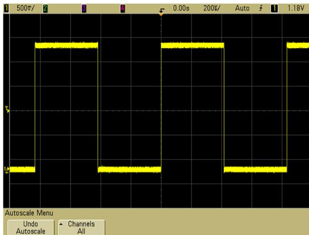
If you see the waveform, but the square wave is not shaped correctly as shown above, perform the procedure “[To compensate the oscilloscope probes](#)” on page 23.
