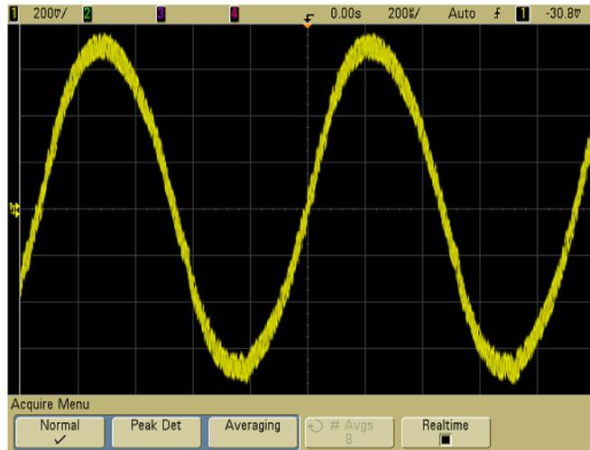
**Figure 39** Random noise on the displayed waveform
