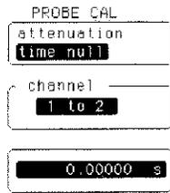
The time null menu sets the timing of all channels to correspond to channel 1 at the probe tip. This eliminates time discrepancies between channels caused by variations in cable lengths. Also, you can use time null to manually adjust for any differences in cable length by horizontally overlaying displayed waveforms that are time-skewed.
