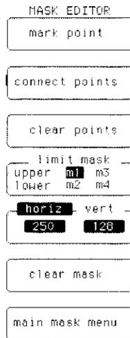
The Mask Editor menu contains the selections used to edit previously generated or stored masks using the automask menu. By using the mask editor menu, it is also possible to clear any existing masks and create a new one using the mark and connect-point method.
