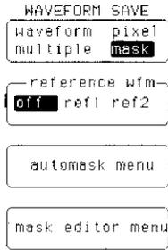
This menu is displayed when mask is selected from the waveform save menu. The mask main menu allows you to view the reference waveforms, or to select the automask or mask editor menus.
