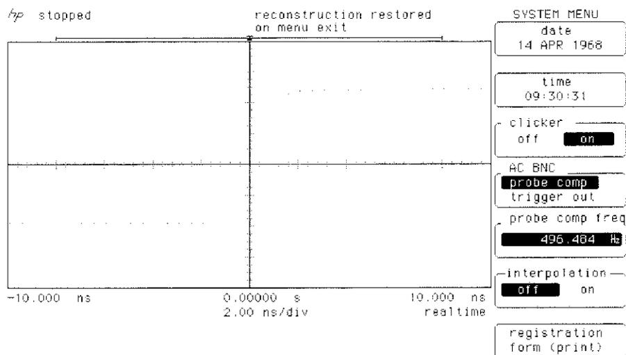
**Single-shot acquisition using the real-time sampling mode and with the interpolator turned off.**
