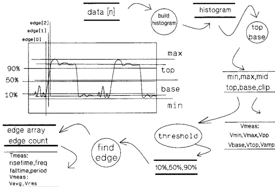
**Thresholds are used to determine edges**
