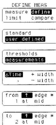
**Measurements** The measurements selection allows you to further customize the +width, -width, and Δtime (delay) measurements. Width measurements allow you to select the threshold (upper, middle, or lower). Where these thresholds occur is defined by the thresholds softkey.
