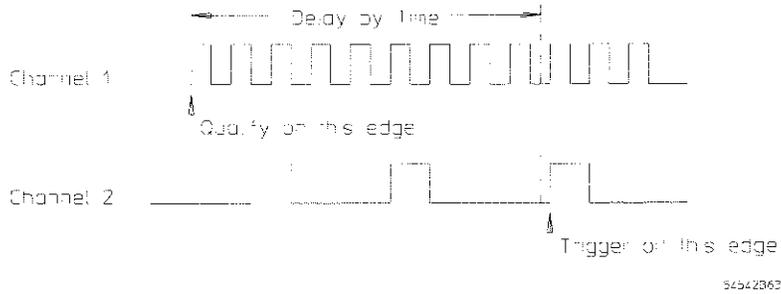
Figure 5-12 shows a delay-by-events timing diagram. You may notice that the qualifying event is channel 1, and the trigger event is channel 2. By changing the number of events, you can consecutively look at pulses in a pulse burst without the effects of jitter. After the number of events are counted, the scope triggers on the edge number you select.
