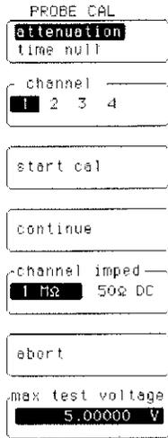
The attenuation menu calibrates the channel gain to the tip of the probe on high impedance probes. The oscilloscope calibrates to correct for channel gain through probe attenuation down to a 0.9 attenuation factor.
