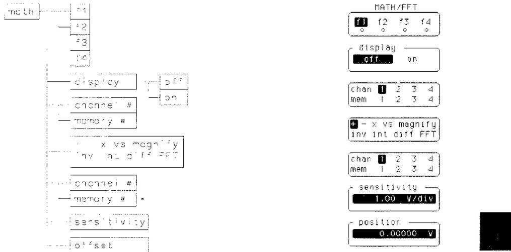
\* The second channel # memory # operand is only available with the  $\times$ ,  $\div$ ,  $\times$ , and vs operators
