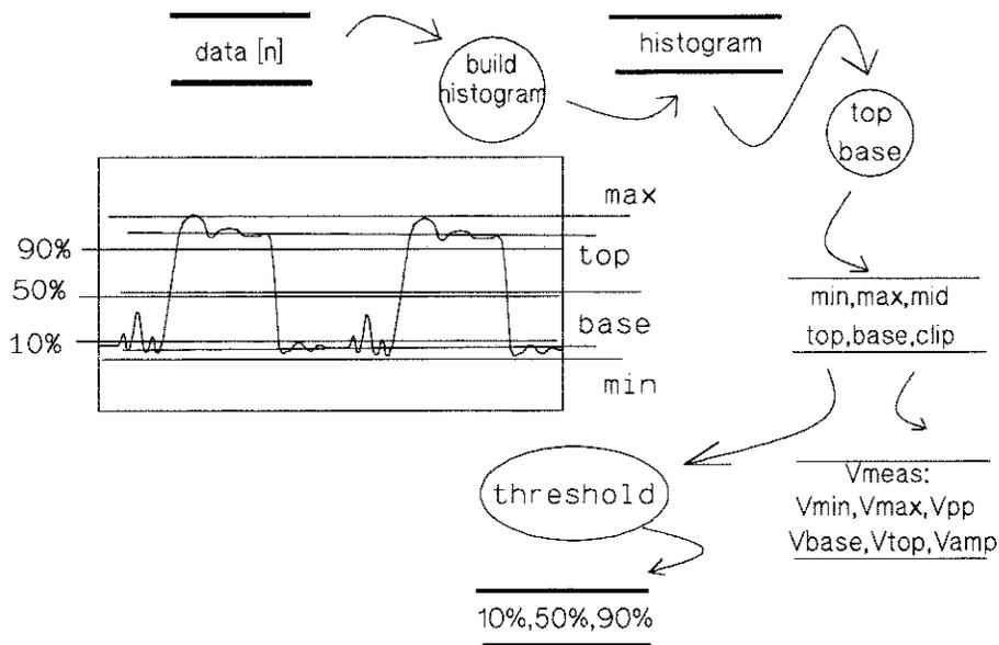
**The oscilloscope calculates the 10, 50, and 90 percent thresholds**
