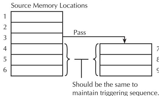
Caution must be used when branching since infinite memory loops can inadvertently be created. Also, a single Source Memory Sweep will always sweep the number of points specified, regardless of how many branches were taken.
