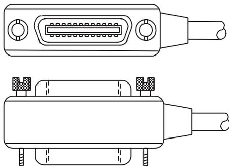
To allow many parallel connections to one instrument, stack the connectors. Two screws are located on each connector to ensure that connections remain secure. Present standards call for metric threads, which are identified with dark-colored screws. Earlier versions have different screws, which are silver-colored. Do not use these types of connectors on the SourceMeter; it is designed for metric threads.
