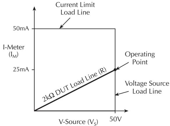
$$\begin{aligned} I_M &= V_S / R \\ &= 50V / 2k\Omega \\ &= 25mA \end{aligned}$$
