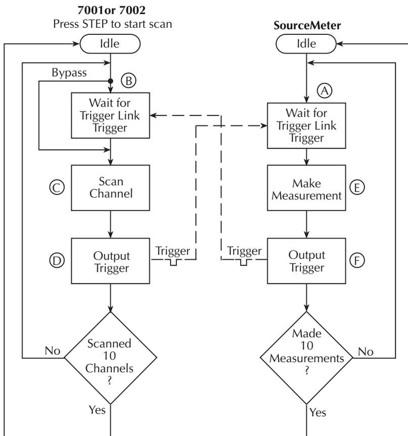
A) Turning the SourceMeter OUTPUT ON places it at point A in the flowchart, where it waits for an external trigger.
