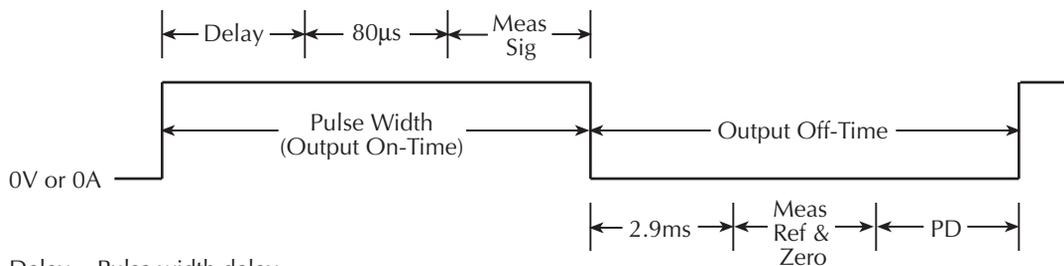
Delay = Pulse width delay
