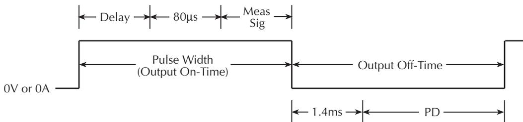
Delay = Pulse width delay
