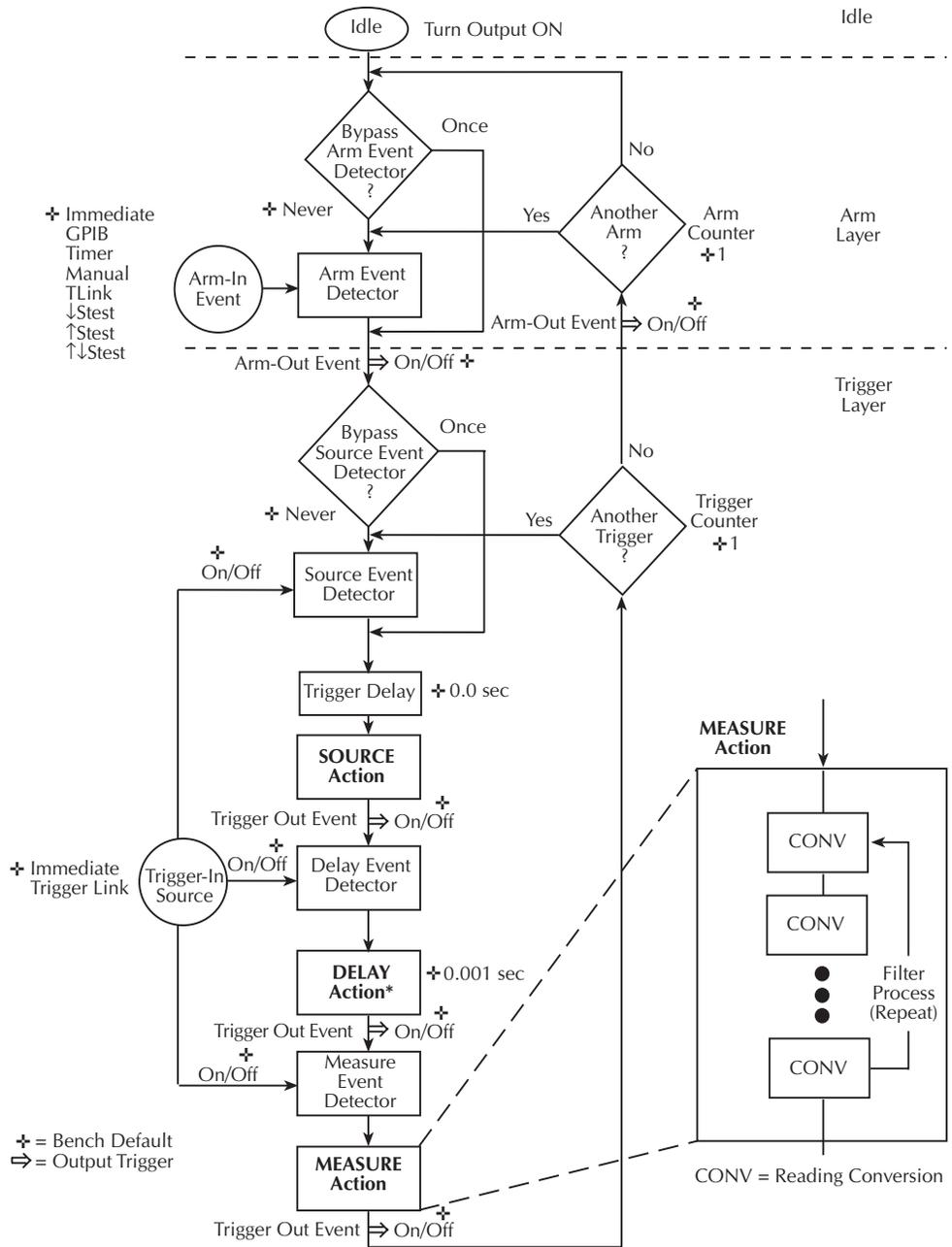
\* Soak time takes the place of the delay time only during the first SDM cycle after initial sweep trigger if the unit is in the MULTIPLE mode. See Section 7, "Autorange change mode."
