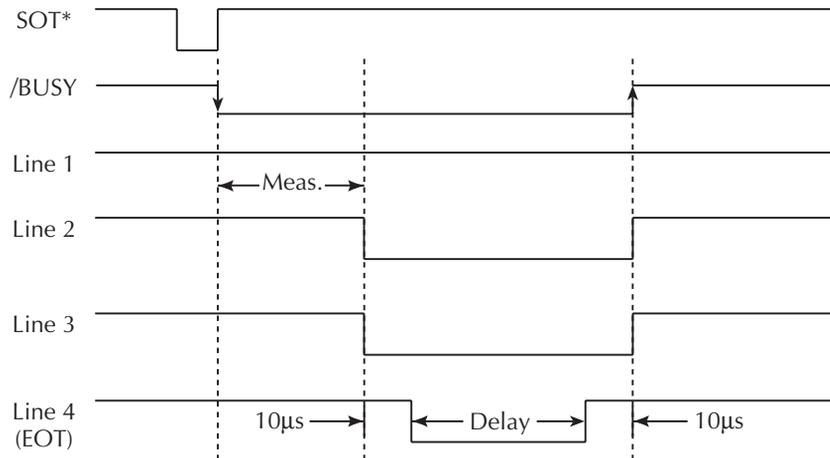
\* With the SOT line being pulsed low (as shown),  $\downarrow$ STEST must be the selected event for the trigger model. If the SOT line is instead pulsed high by the handler,  $\uparrow$ STEST must be the selected arm event. For high or low pulses, select  $\uparrow\downarrow$ STEST.
