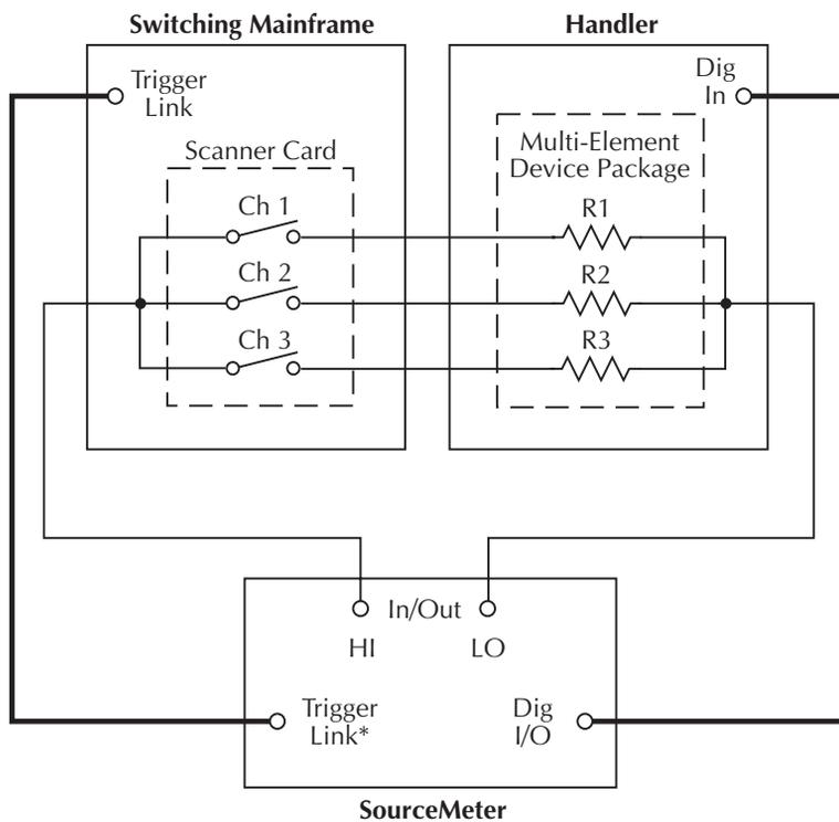
\*Trigger layer configured to output trigger pulse after each measurement.
