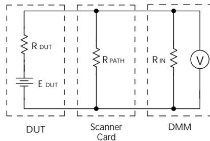
$R_{DUT}$  = Source Resistance of DUT
