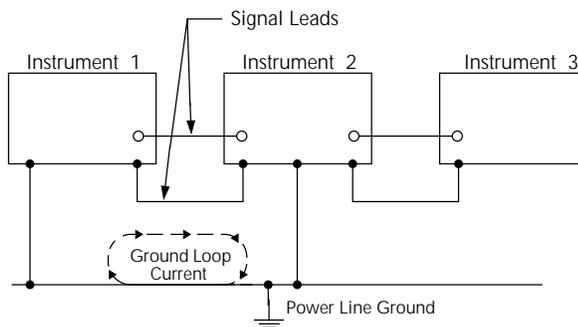
Figure 3-8 shows how to connect several instruments together to eliminate this type of ground loop problem. Here, only one instrument is connected to power line ground. Ground loops are not normally a problem with instruments having isolated LO terminals. However, all instru-
