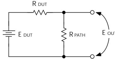
$$E_{OUT} = \frac{E_{DUT} R_{PATH}}{R_{DUT} + R_{PATH}}$$
