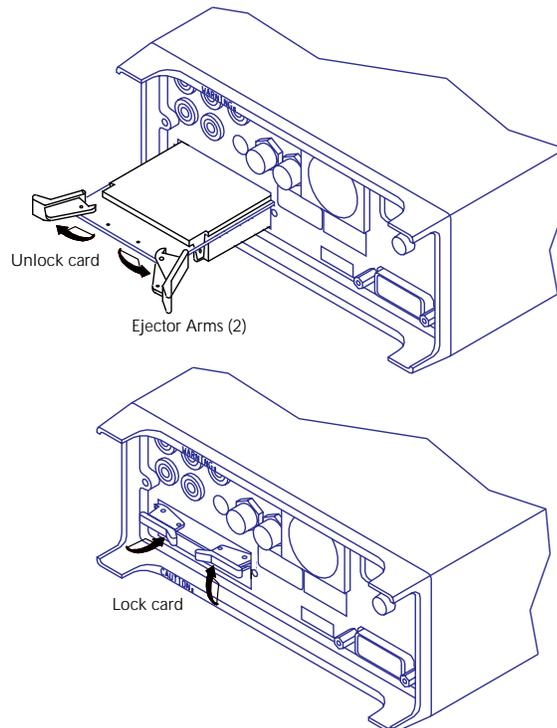
Note: Card installation in a Model 2001/2002 is shown. For installation in Model 2000, turn card over.
