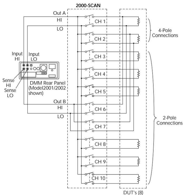
Measurement functions for each scanner channel are defined using the INTERNAL-CHANS menu available by pressing CONFIG-CHAN (see "Using the scanner with the buffer"). Measurement functions for this test would be set up as follows:
