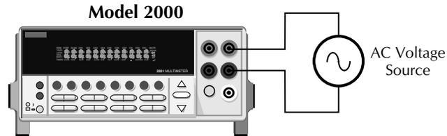
Input Impedance =  $1\text{M}\Omega$  in parallel with  $<100\text{pF}$
