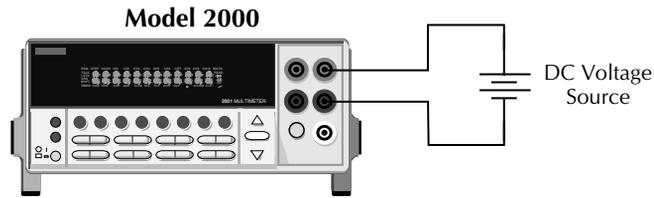
Input Resistance =  $10\text{M}\Omega$  on 1000V and 100V ranges ;
