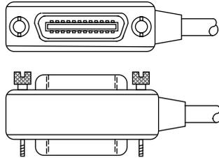
To allow many parallel connections to one instrument, stack the connector. Two screws are located on each connector to ensure that connections remain secure. Current standards call for metric threads, which are identified with dark-colored screws. Earlier versions had different screws, which were silver-colored. Do not use these types of connectors on the Model 2000 multimeter, because it is designed for metric threads.
