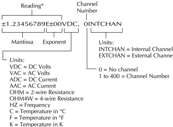
\* An overflow reading is displayed as +9.9E37 with no units
