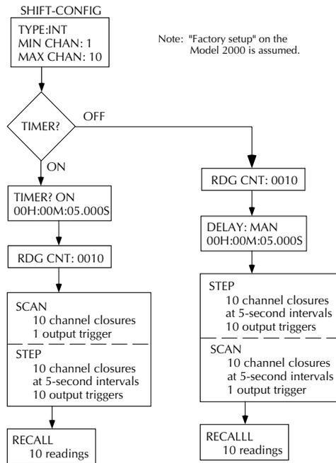
When using both the timer and delay parameters, the timer is not started until after the delay. For example, if the timer is two minutes and the delay is ten seconds, the timer is not started until 10sec after pressing SCAN. Each successive scan will occur at 2:10.0, 4:10.0, etc.
